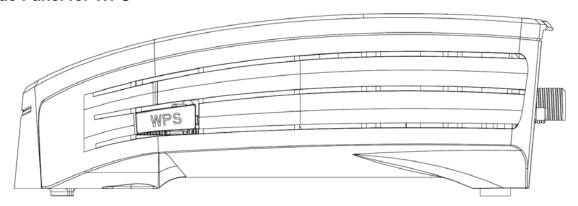
WPS button: Wi-Fi Protected Setup<sup>TM</sup>. This button can be used to:
