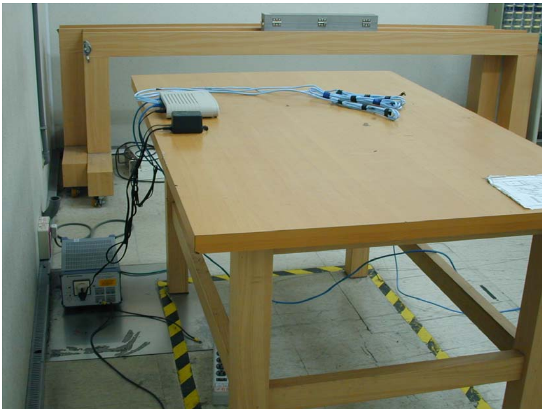
Back View of Conducted Test (Mode 1)
