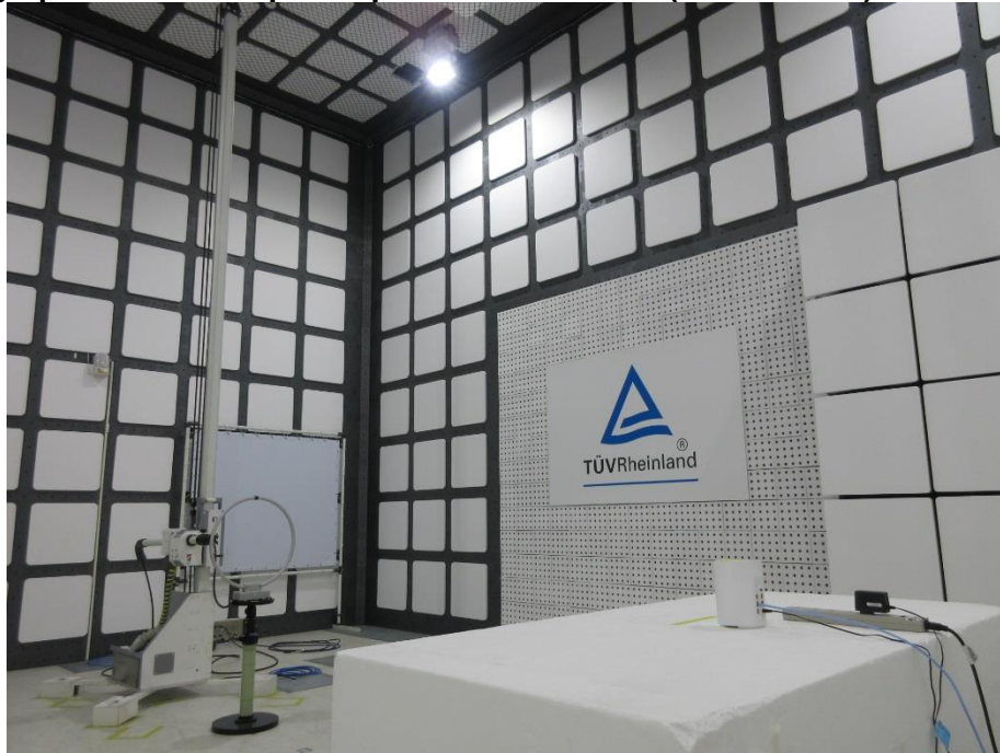
Photograph 3: Test Setup for Spurious Emissions (Back View 1)
