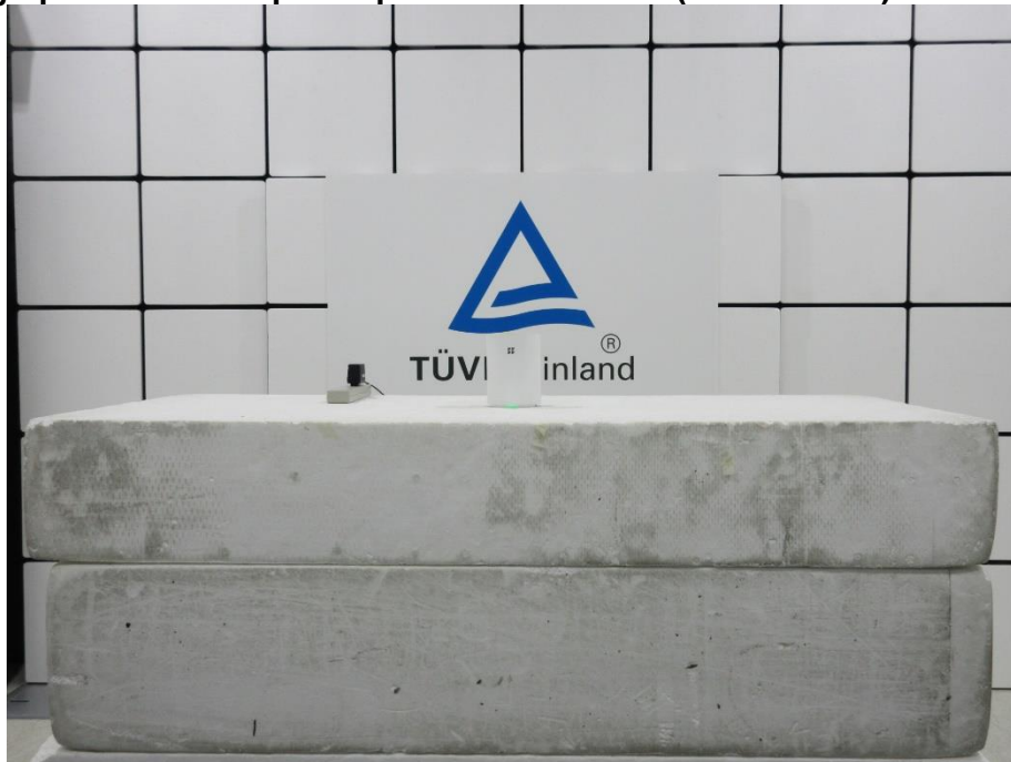
Photograph 2: Test Setup for Spurious Emissions (Front View 2)
