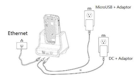
Left LED blinks in red indicating low and risk battery and stating red indicating that the battery is charging. the LED becomes green when battery is fully charged, then.
