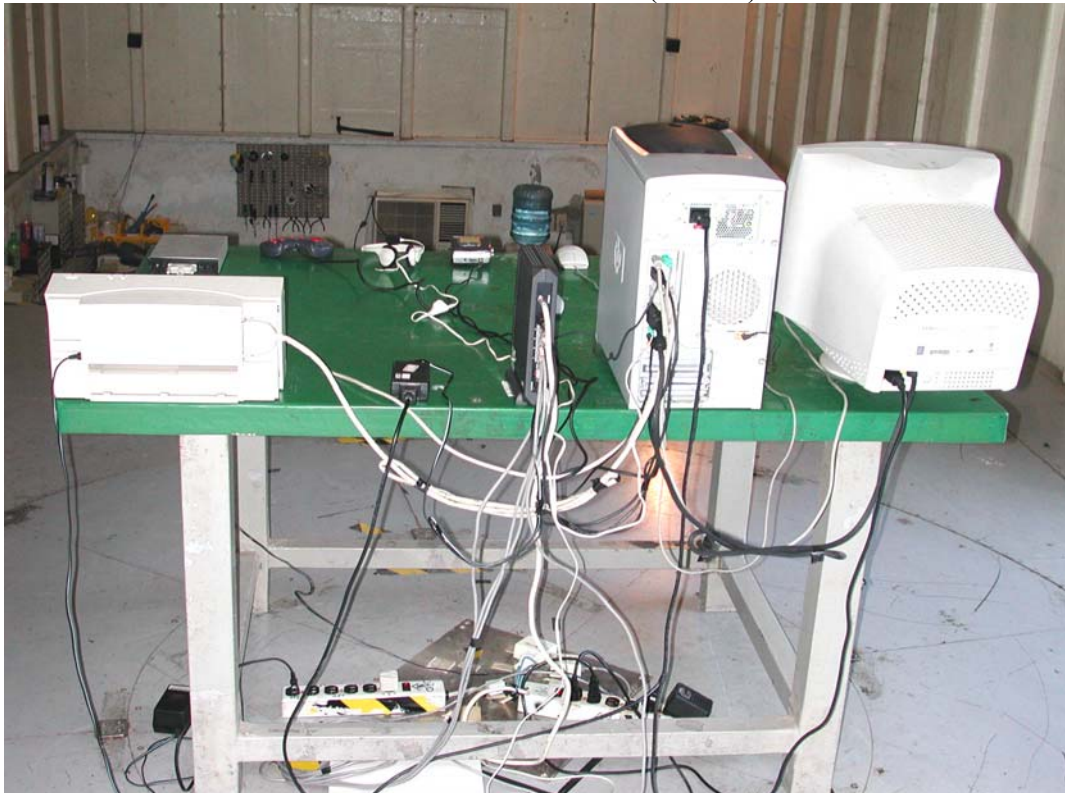
Back View of Radiated Test (Mode 2)
