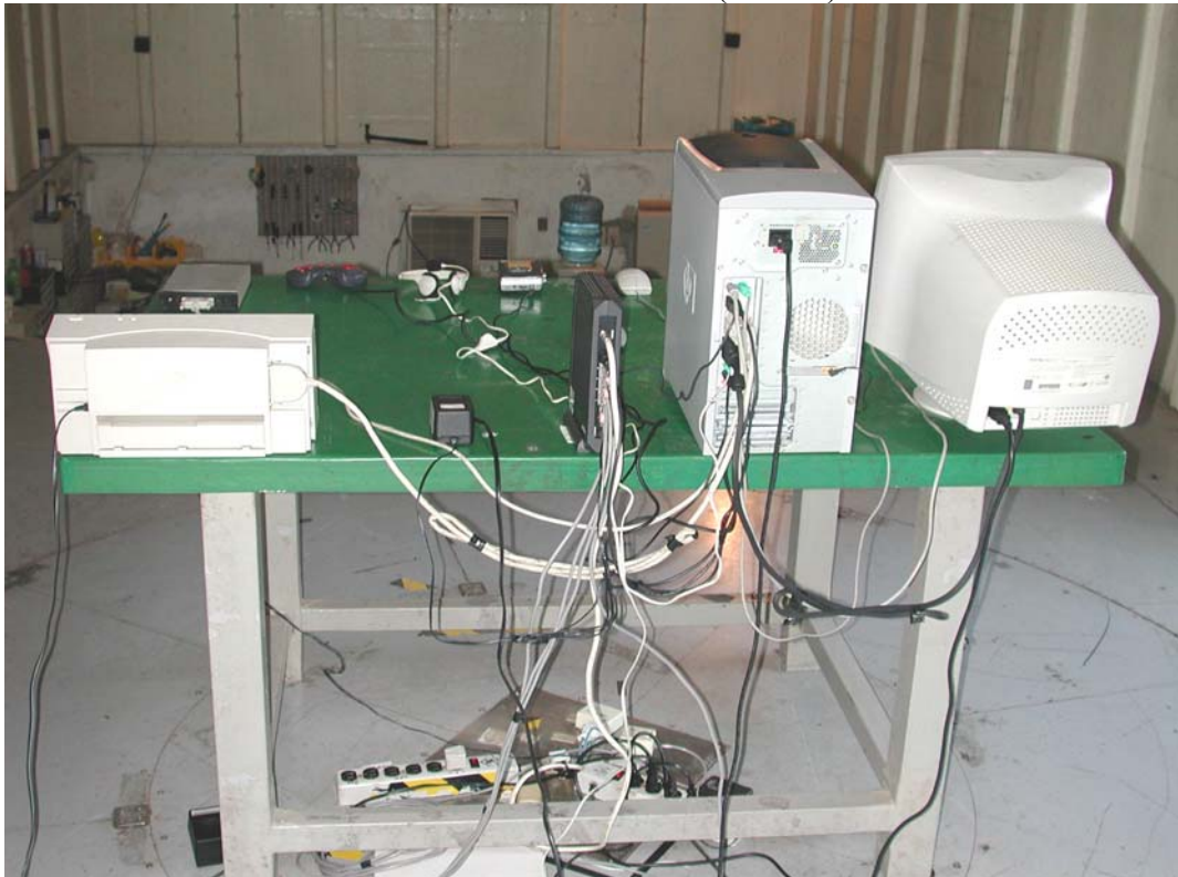
Back View of Radiated Test (Mode 1)
