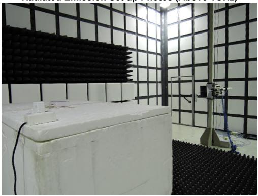
Radiated Emission Set up Photos (Front View)
