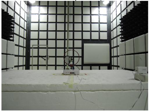
Radiated Emission Set up Photos (Below 1GHz)
