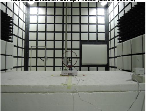
Radiated Emission Set up Photos (Below 1GHz)
