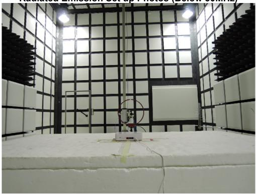
Radiated Emission Set up Photos (Below 1GHz)
