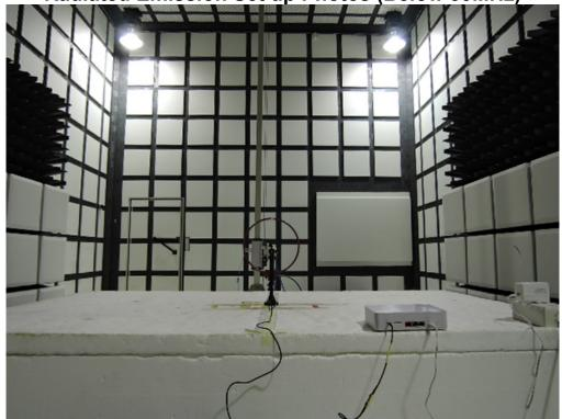
Radiated Emission Set up Photos (Below 1GHz)
