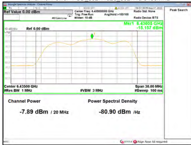
Channel Power+PSD_802.11a20_802.11a 6475MHz
