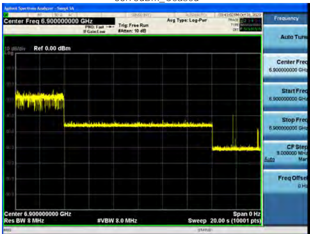
802.11be_320MHz_CF 6745MHz_Interference_6900MHz_-69.73dBm_Mini- mal
