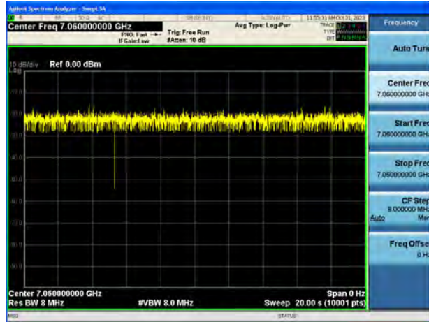
802.11be_320MHz_CF 6905MHz_Interference_6905MHz_-76.6dBm_Normal 802.11be_320MHz_CF 6905MHz_Interference_7060MHz_-76.7dBm_Normal
