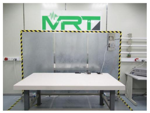
Test Mode: Mode1 Description: Back View of Conducted Emission Test Setup
