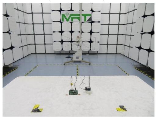
Description: Radiated Spurious Emission Test Setup for  $1\text{GHz} \sim 18\text{GHz}$
