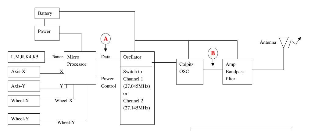
RFW-33 Wireless Radio Wheel Mouse (Transmitter)
