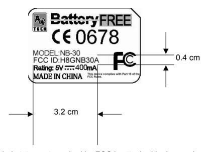
The remained portion of label statement required by FCC is attached in the user's manual.
