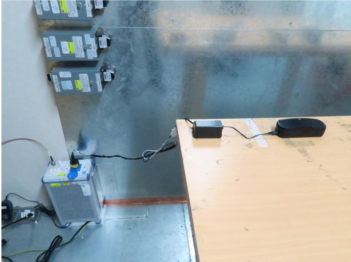
Photograph 6: Set-up for for Mains Conducted testing Front
