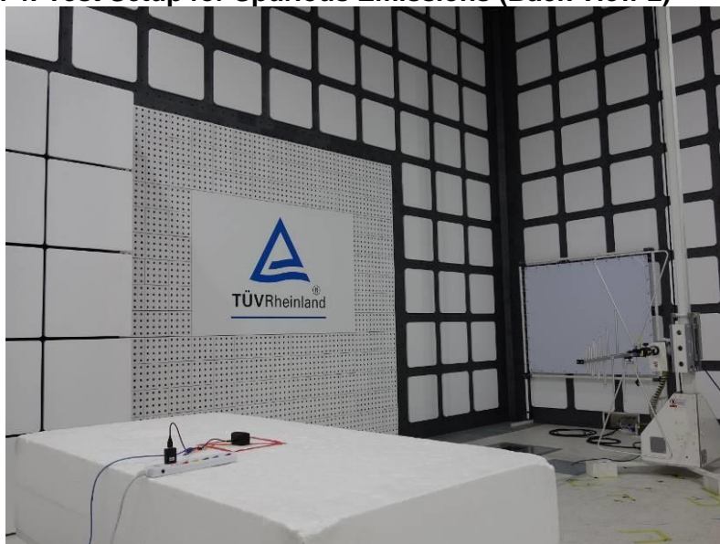
Photograph 4: Test Setup for Spurious Emissions (Back View 2)
