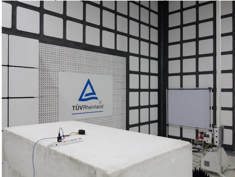
Photograph 6: Test Setup for Spurious Emissions (Back View 4)
