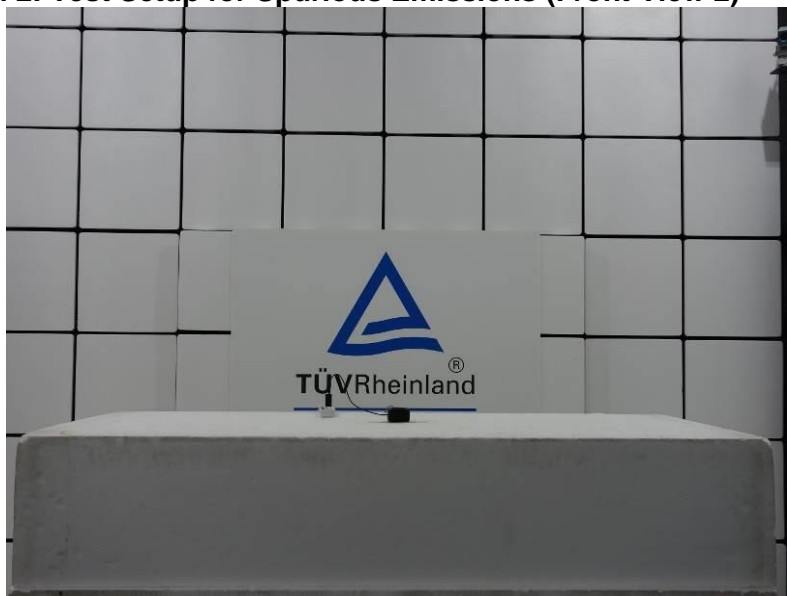
Photograph 2: Test Setup for Spurious Emissions (Front View 2)
