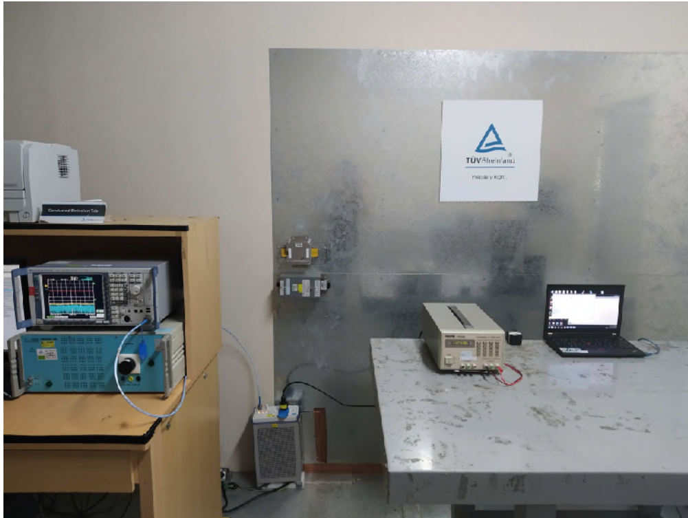
Photograph 7: Set-up for Mains Conducted testing (Front View)
