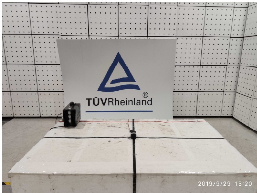
Photograph 1: Set-up for Spurious Emissions (Front View 1)
