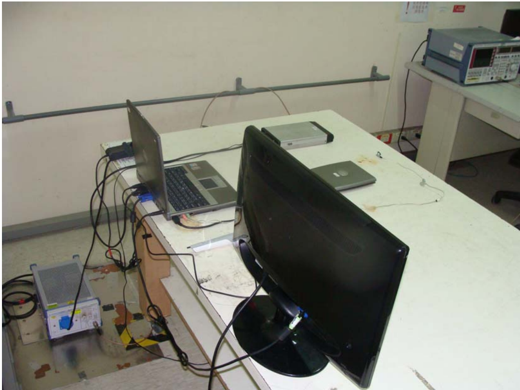
Back View of Spurious Emission Test
