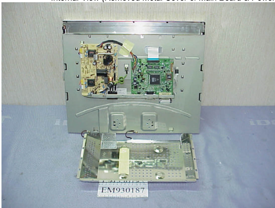
Figure 6 Internal View (Removed Metal Cover of Main Board & Power Board)
