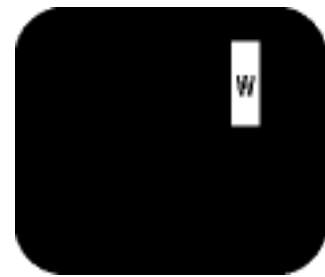
Three adjacent lit subpixels (one white pixel)
