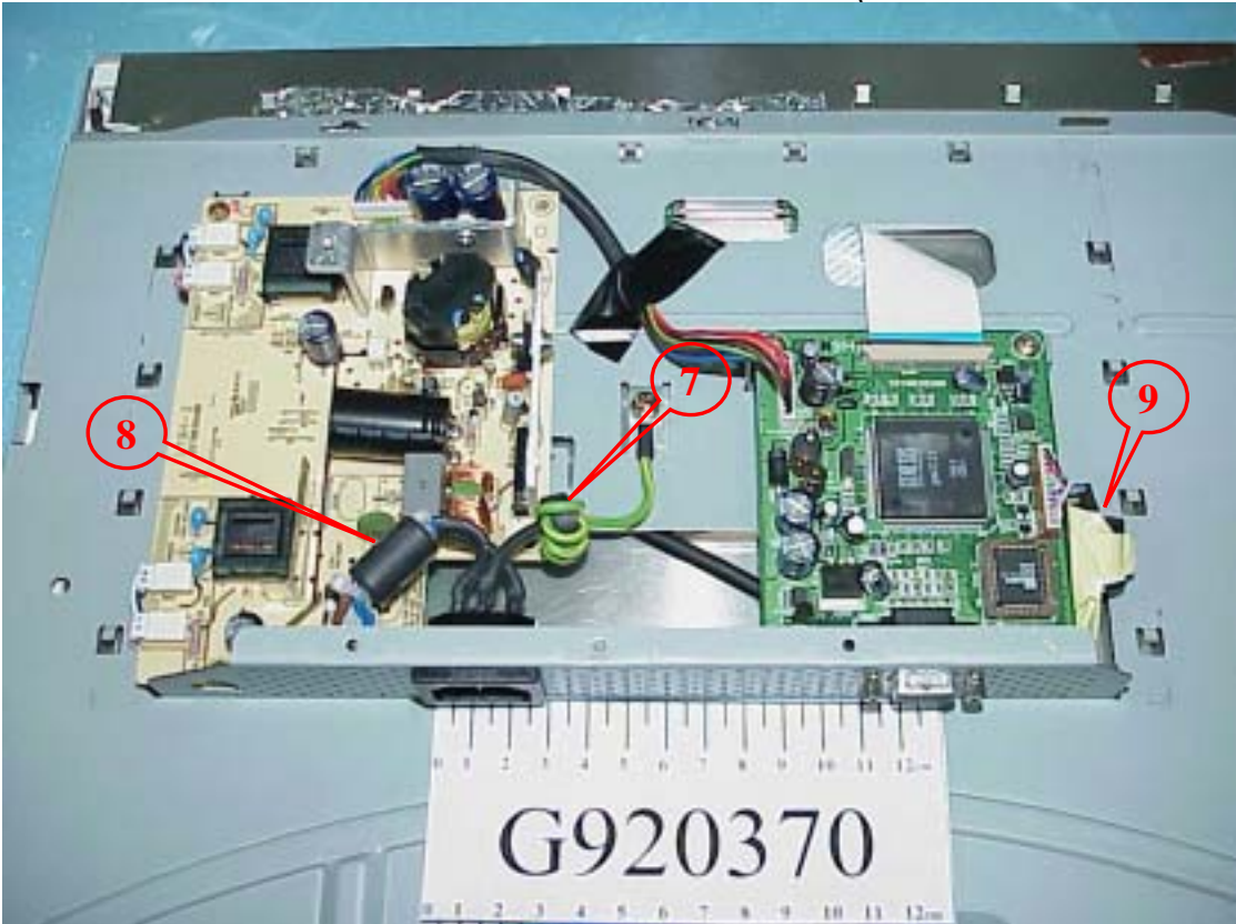
Figure 6 Internal View (Main Board & Power Board)
