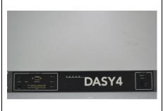
The DASY4/DASY5 measurement server is based on a PC/104 CPU board with a 166MHz low-power Pentium, 32MB chip disk and 64MB RAM. The necessary circuits for communication with either the DAE3 electronic box as well as the 16-bit AD-converter system for optical detection and digital I/O interface are contained on the DASY4/DASY5 I/O-board, which is directly connected to the PC/104 bus of the CPU board.
