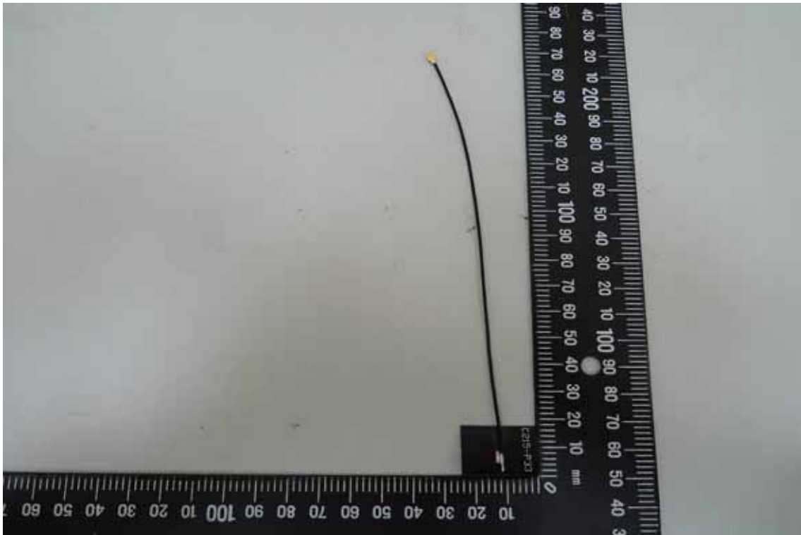
WLAN Antenna – 1 (PIFA Antenna, Model No.: RFA-02-P33-70B-150)
