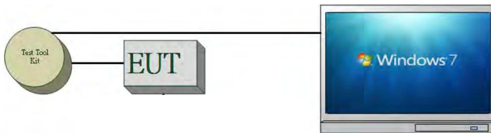
Fig. 2-1 AC Power Line Conducted Emission Configuration
