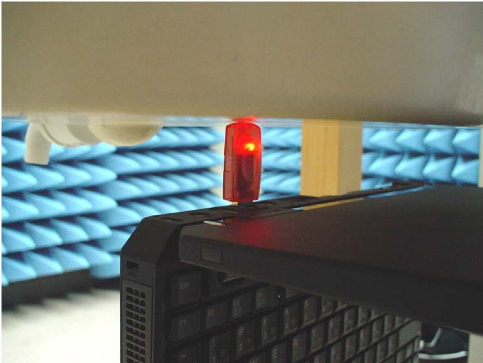
Fig.3 Photograph of the antenna tip is upward and at a distance of 0.0 cm from the base of the phantom.
