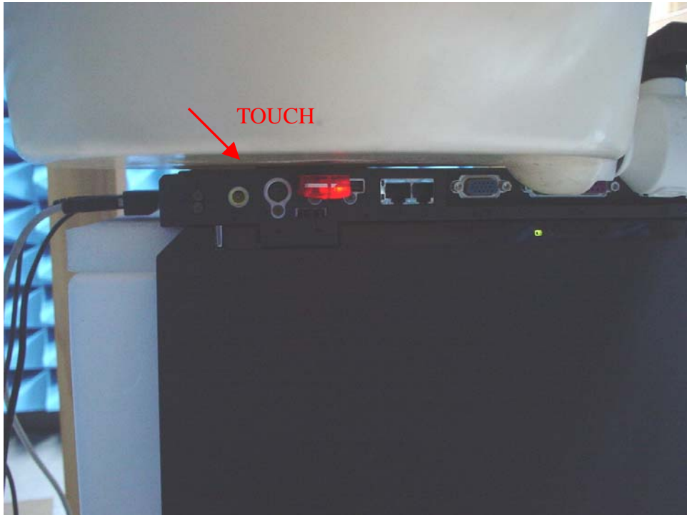
Fig.7 Photograph of the Bottom of the Pc is paralleled and at a distance of 0.0 cm from the base of the phantom.
