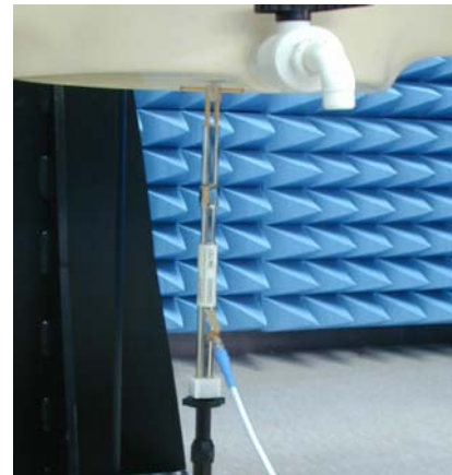
Photograph of the 2450MHz System Check
