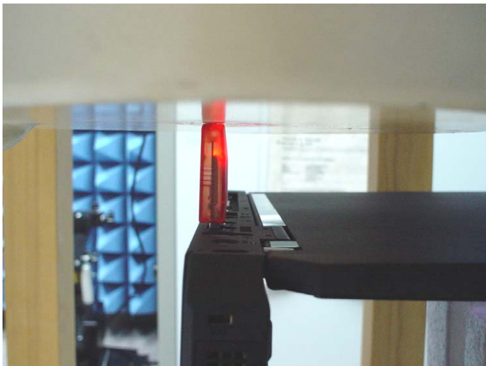
Fig.4 Photograph of the antenna tip is upward and at a distance of 0.0 cm from the base of the phantom.
