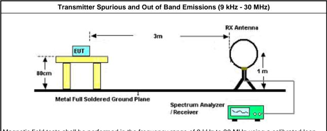
Magnetic field tests shall be performed in the frequency range of 9 kHz to 30 MHz using a calibrated loop antenna.
