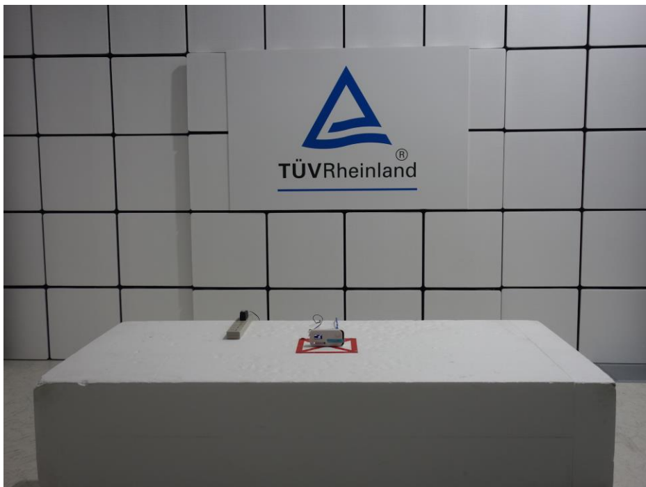
Photograph 2: Set-up for Spurious Emissions (Front View 2)
