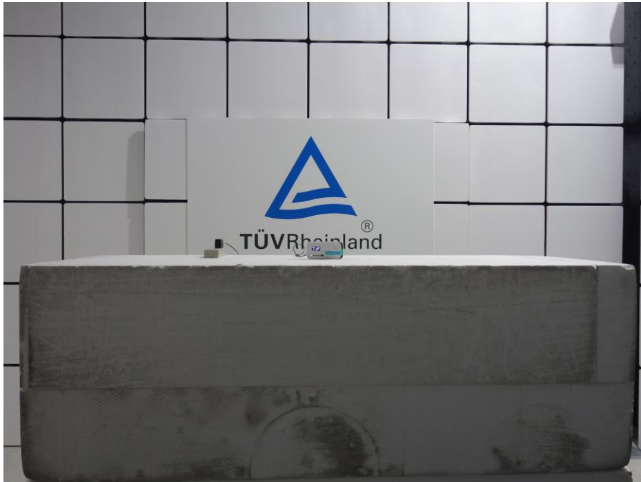
Photograph 1: Set-up for Spurious Emissions (Front View 1)
