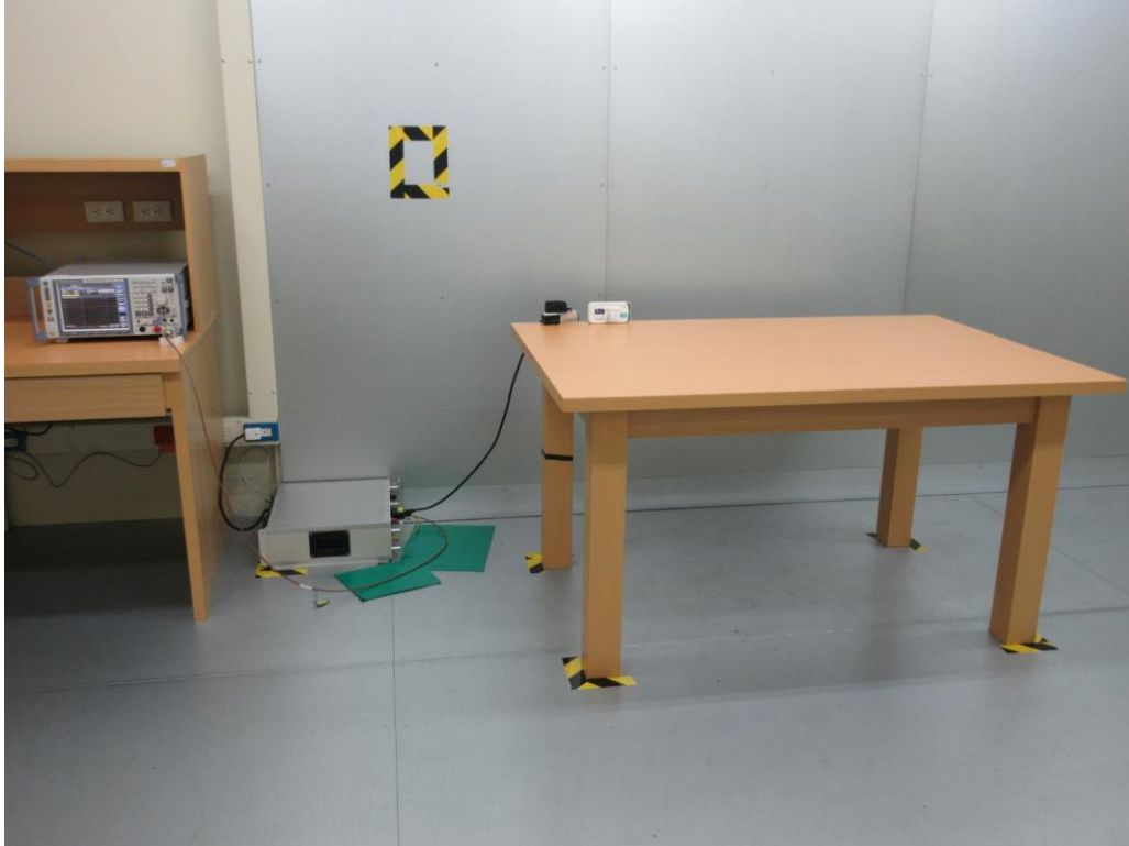
Photograph 7: Set-up for AC Mains (Front View)
