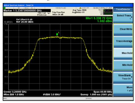
802.11n(40M) (5.15GHz-5.25GHz) The Lowest Channel 38: 5190MHz
