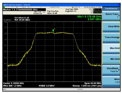
802.11a (5.15GHz-5.25GHz) The Middle Channel 40: 5200MHz
