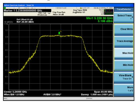
802.11n(20M) (5.15GHz-5.25GHz) The Lowest Channel 36: 5180MHz
