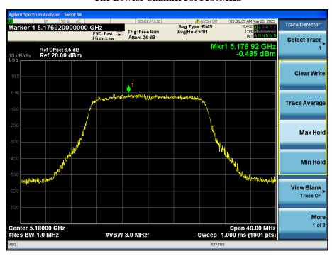
802.11ac (5.15GHz-5.25GHz) The Middle Channel 40: 5200MHz
