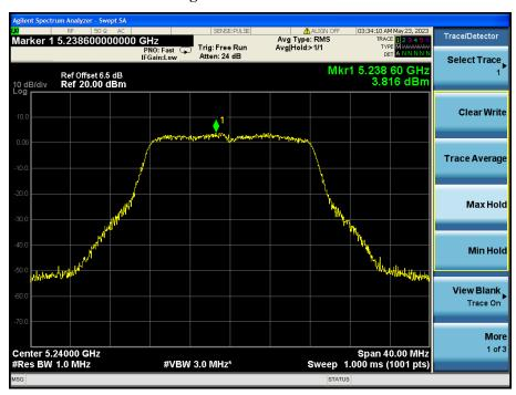
802.11n(20M) (5.15GHz-5.25GHz) The Lowest Channel 36: 5180MHz
