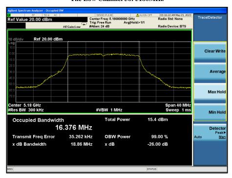
802.11a (5.15GHz-5.25GHz) The Middle Channel 40: 5200MHz
