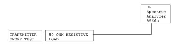
METHOD OF MEASUREMENT: The procedure used was TIA/EIA-603 STANDARD without any exceptions. The measurements were made at TIMCO ENGINEERING INC. 849 N.W. State Road 45, Newberry, Florida 32669.
