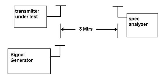
METHOD OF MEASUREMENTS: The tabulated data shows the results of the radiated field strength emissions test. The spectrum was scanned from 30 MHz to at least the tenth harmonic of the fundamental. This test was conducted per TIA/EIA STANDARD 603 using the substitution method. Measurements were made at the open field test site of TIMCO ENGINEERING, INC. located at 849 NW State Road 45, Newberry, FL 32669.
