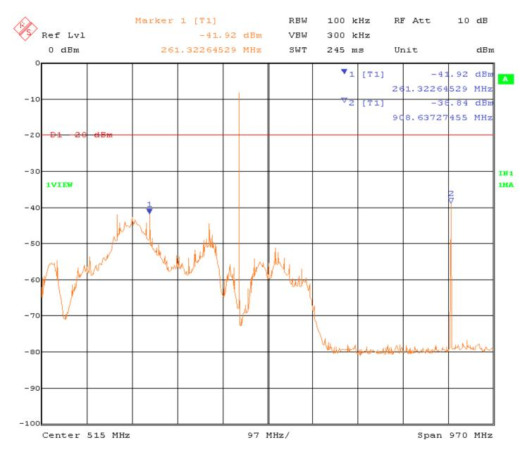
Note: For this test, a band-reject filter was applied to the fundamental frequency.
