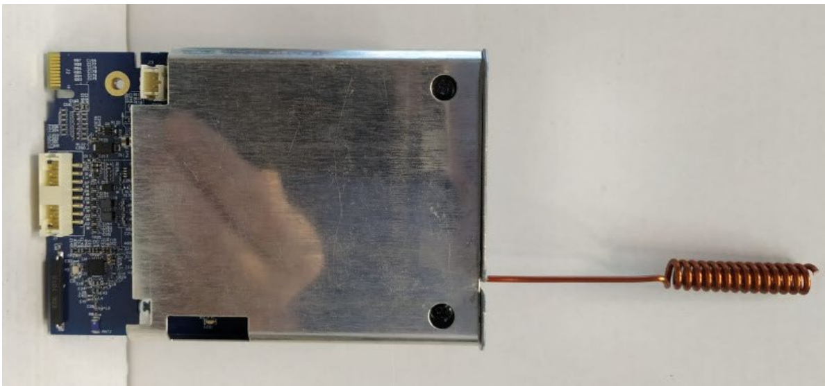
PCB front, with Shield and Antenna
