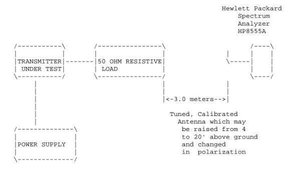
Equipment placed 4' above ground on a rotatable platform.
