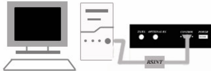
Figure 9: BSR100D/PC Connection Configuration
