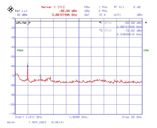
Plot # 43: Transmitter Conducted Emissions Outside the Permitted Band Frequency: 1880 MHz, Modulation: GSM
