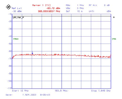
Plot # 30 : Transmitter Conducted Emissions Outside the Permitted Band Frequency: 1851 MHz, Modulation: CDMA
