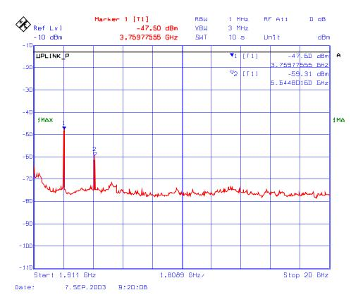
Plot # 33 : Transmitter Conducted Emissions Outside the Permitted Band Frequency: 1909 MHz, Modulation: CDMA
