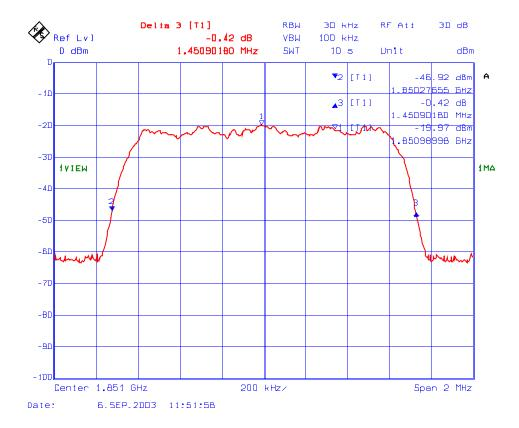
Plot # 13 : 26 dB BW of the 1850 – 1910 MHz, RF Output Frequency: 1880 MHz, Modulation: CDMA
