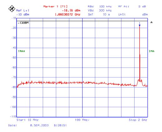
**Plot # 50 :** Transmitter Conducted Emissions (Multiple Channel Inputs/Outputs)
