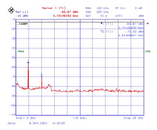
Plot # 53 : Transmitter Conducted Emissions (Multiple Channel Inputs/Outputs) In 1850 – 1910 MHz Band
