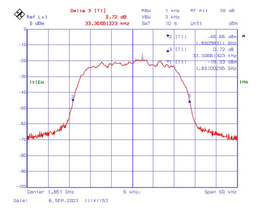
Plot # 17 : 26 dB BW of the 1850 – 1910 MHz, RF Output Frequency: 1880 MHz, Modulation: TDMA
