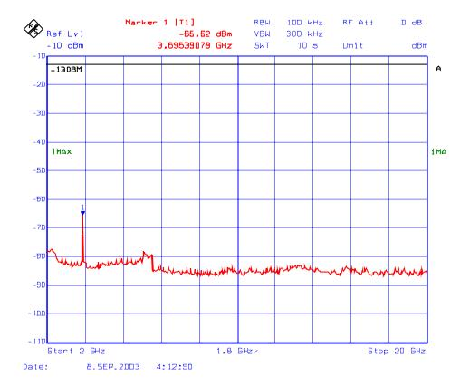
Plot # 49 : Transmitter Conducted Emissions (Multiple Channel Inputs/Outputs) In 1850 – 1910 MHz Band
