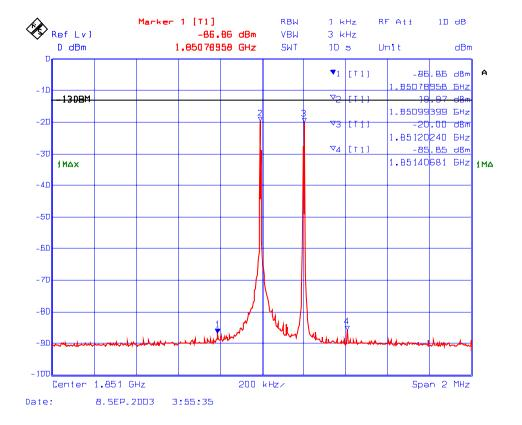
RF Input 1: -49.35 dBm, RF Input 2: -49.35 dBm, RF Input 3: -49.35 dBm
