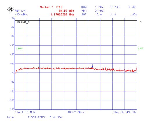
Plot # 44 : Transmitter Conducted Emissions Outside the Permitted Band Frequency: 1880 MHz, Modulation: GSM
