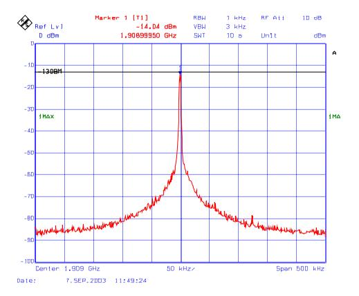
Plot # 8: RF Output Power with 2 RF signal input/output in 1850 – 1910 MHz
