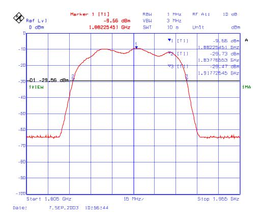
Plot # 11 : 26 dB BW of the 1850 – 1910 MHz, RF Input Frequency: 1880 MHz, Modulation: CDMA
