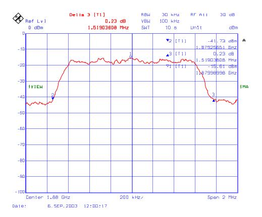
Plot # 14 : 26 dB BW of the 1850 – 1910 MHz, RF Output Frequency: 1909 MHz, Modulation: CDMA
