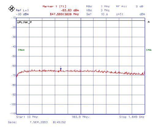
Plot # 40 : Transmitter Conducted Emissions Outside the Permitted Band Frequency: 1909 MHz, Modulation: TDMA
