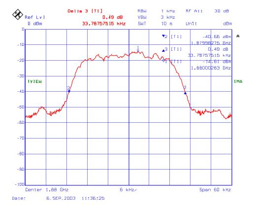
Plot # 18 : 26 dB BW of the 1850 – 1910 MHz, RF Output Frequency: 1909 MHz, Modulation: TDMA
