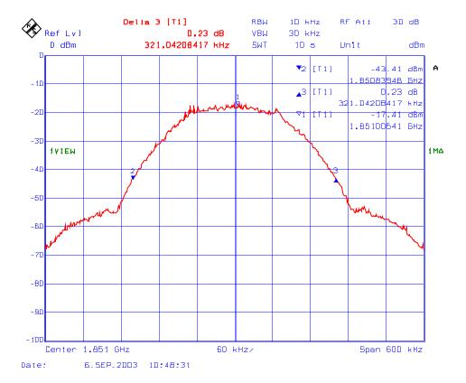
Plot # 21: 26 dB BW of the 1850 – 1910 MHz, RF Output
