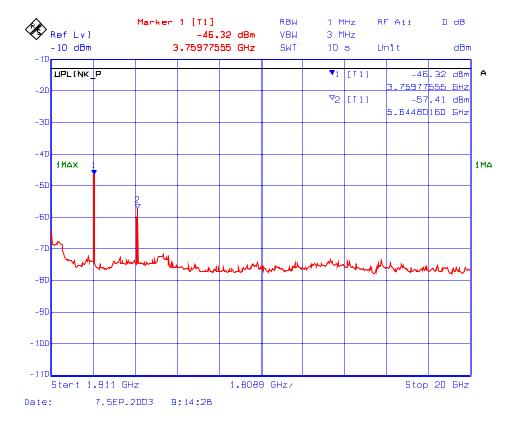
Plot # 39 : Transmitter Conducted Emissions Outside the Permitted Band Frequency: 1909 MHz, Modulation: TDMA
