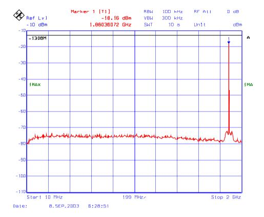
Plot # 54 : Transmitter Conducted Emissions (Multiple Channel Inputs/Outputs) In 1850 – 1910 MHz Band
