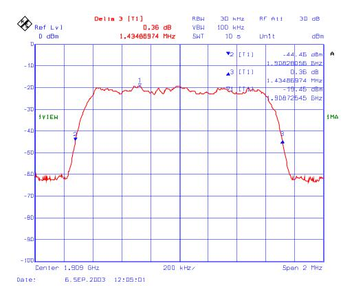
Plot # 15 : 26 dB BW of the 1850 – 1910 MHz, RF Input Frequency: 1880 MHz, Modulation: TDMA
