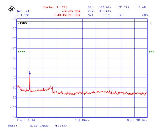
Plot # 57 : Transmitter Conducted Emissions (Multiple Channel Inputs/Outputs) In 1850 – 1910 MHz Band
