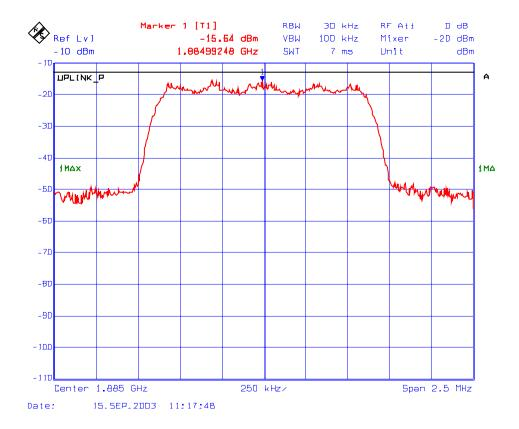
Block 4, Upper Band-Edge Conducted Emissions Frequency: 1890 MHz, Modulation: CDMA
