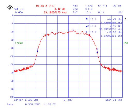
Plot # 19: 26 dB BW of the 1850 – 1910 MHz, RF Input Frequency: 1880 MHz, Modulation: GSM
