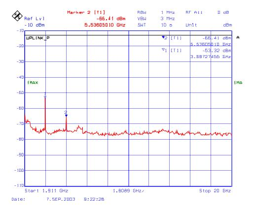
Plot # 31 : Transmitter Conducted Emissions Outside the Permitted Band Frequency: 1880 MHz, Modulation: CDMA
