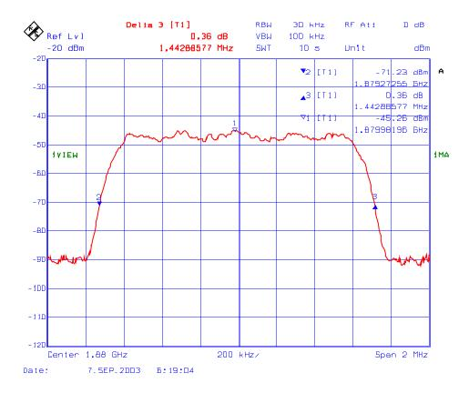
Plot # 12 : 26 dB BW of the 1850 – 1910 MHz, RF Output Frequency: 1851 MHz, Modulation: CDMA
