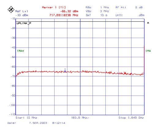
Plot # 42 : Transmitter Conducted Emissions Outside the Permitted Band Frequency: 1851 MHz, Modulation: GSM
