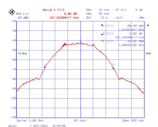
Plot # 20 : 26 dB BW of the 1850 – 1910 MHz, RF Output
