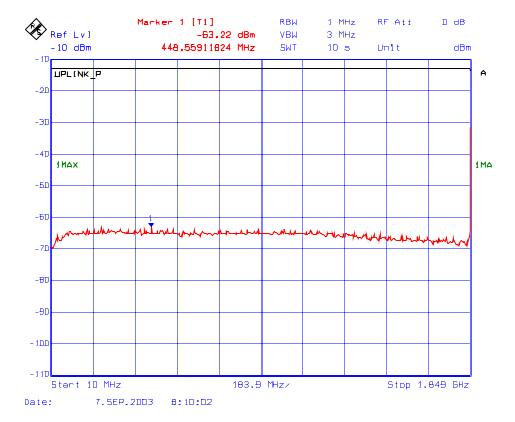
Plot # 36 : Transmitter Conducted Emissions Outside the Permitted Band Frequency: 1851 MHz, Modulation: TDMA
