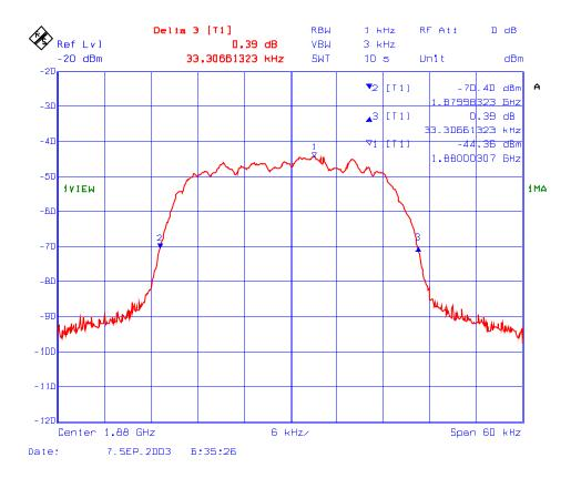
Plot # 16 : 26 dB BW of the 1850 – 1910 MHz, RF Output Frequency: 1851 MHz, Modulation: TDMA
