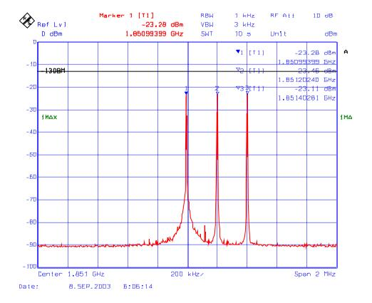
Plot # 4: RF Output Power with 1 RF signal input/output in 1850 – 1910 MHz Fc: 1880 MHz, RF Input: -40 dBm
