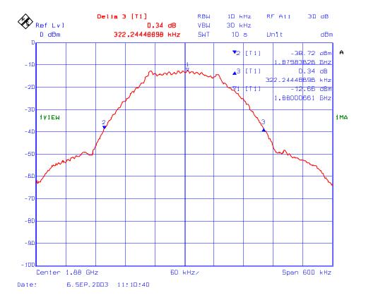
Plot # 22 : 26 dB BW of the 1850 – 1910 MHz, RF Output Frequency: 1909 MHz, Modulation: GSM
