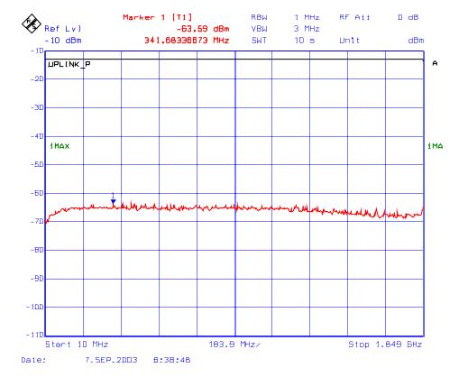
Plot # 38 : Transmitter Conducted Emissions Outside the Permitted Band Frequency: 1880 MHz, Modulation: TDMA
