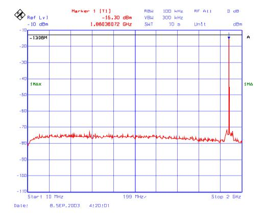
Plot # 52 : Transmitter Conducted Emissions (Multiple Channel Inputs/Outputs) In 1850 – 1910 MHz Band
