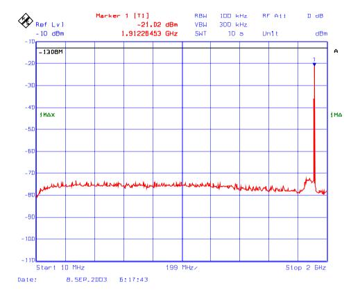
Plot # 58 : Transmitter Conducted Emissions (Multiple Channel Inputs/Outputs) In 1850 – 1910 MHz Band
