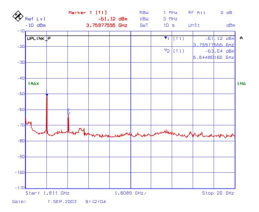
Plot # 45 : Transmitter Conducted Emissions Outside the Permitted Band Frequency: 1909 MHz, Modulation: GSM
