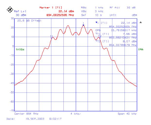
PLOT # 114 99% Occupied Bandwidth- RF Input
