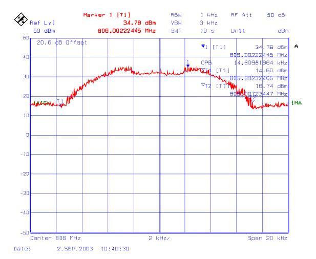
PLOT # 65 99% Occupied Bandwidth-RF Output
