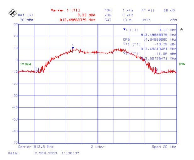
**PLOT #63** 99% Occupied Bandwidth- RF Output Frequency: 813.5 MHz, 25 kHz Channel Spacing Modulation: FM modulation with an external 9600 b/s random data source
