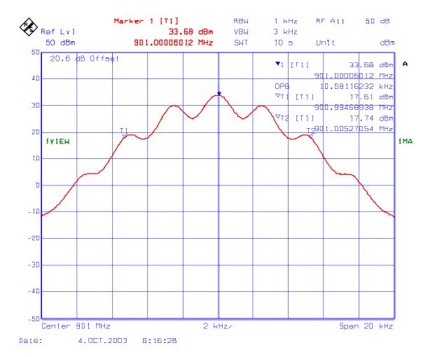
PLOT # 133 99% Occupied Bandwidth- RF Input Frequency: 896 MHz, 12.5 kHz Channel Spacing Modulation: FM modulation with an external 9600 b/s random data source
