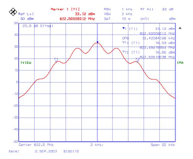
PLOT # 68 99% Occupied Bandwidth-RF Output Frequency: 822.5 MHz, 12.5 kHz Channel Spacing Modulation: FM modulation with 2.5 kHz Sine wave signal
