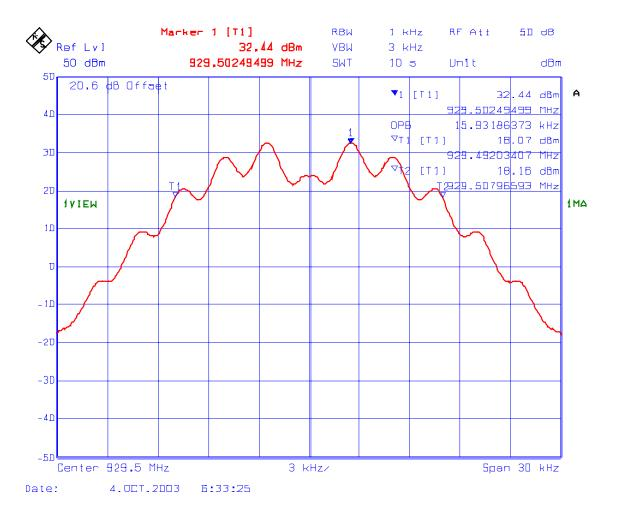
PLOT # 138 99% Occupied Bandwidth- RF Output
