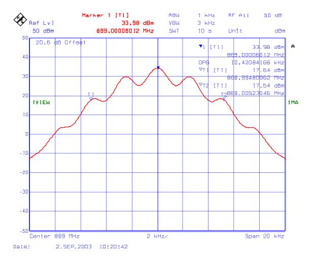
PLOT # 106 99% Occupied Bandwidth- RF Input
