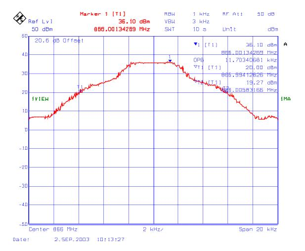
PLOT # 109 99% Occupied Bandwidth- RF Output
