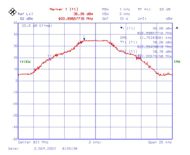
**PLOT #73** 99% Occupied Bandwidth-RF Output Frequency: 824 MHz, 12.5 kHz Channel Spacing Modulation: FM modulation with an external 9600 b/s random data source
