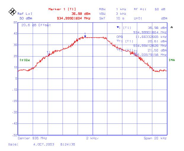
PLOT # 142 99% Occupied Bandwidth- RF Input
