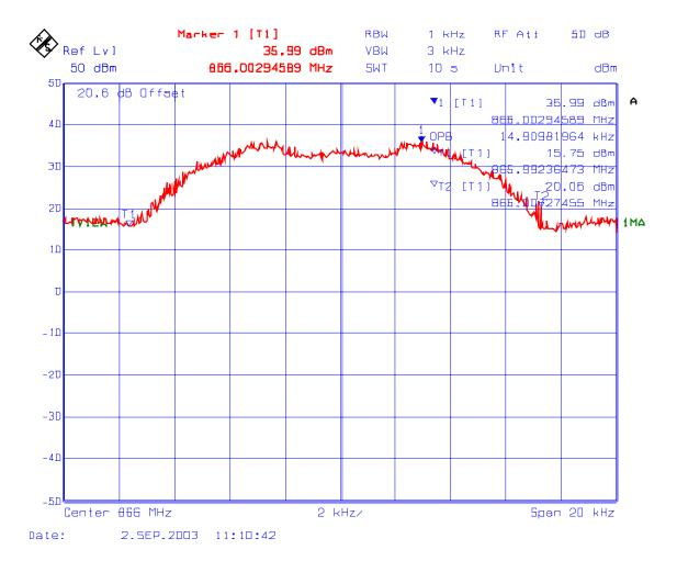
PLOT # 102 99% Occupied Bandwidth- RF Input Frequency: 866 MHz, 12.5 kHz Channel Spacing Modulation: FM modulation with 2.5 kHz Sine wave signal
