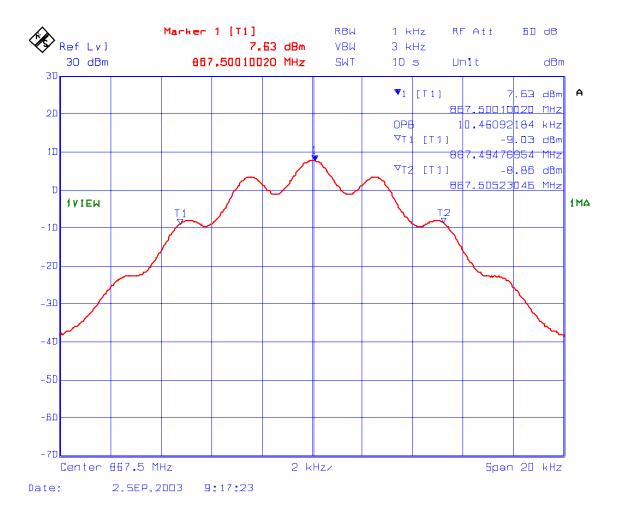
PLOT # 103 99% Occupied Bandwidth- RF Output
