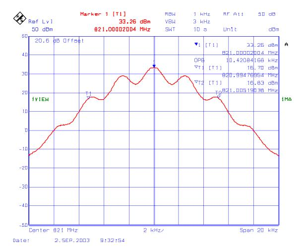
PLOT # 69 99% Occupied Bandwidth-RF Output
