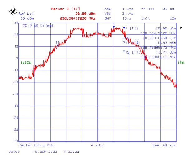
PLOT # 80 99% Occupied Bandwidth- RF Output
