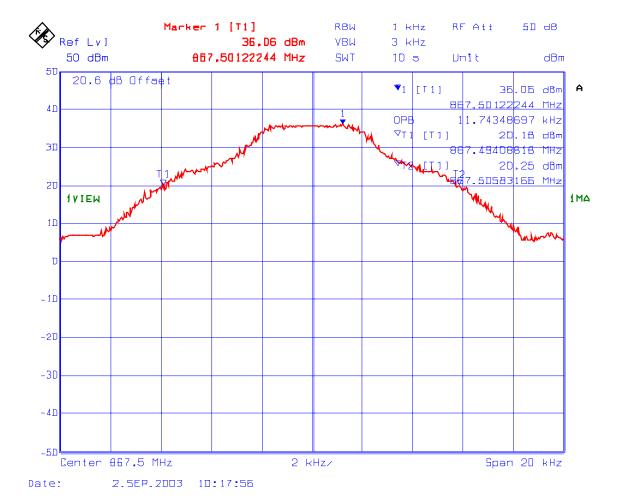
PLOT # 108 99% Occupied Bandwidth- RF Output
