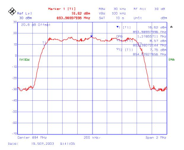
PLOT # 130 99% Occupied Bandwidth- RF Input
