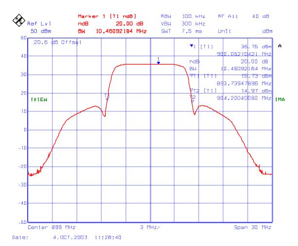
PLOT # 57 20 dB BW of the 928-941 MHz Bandpass Gain RF Input: 10 dBm, Tracking from 900-960 MHz Max Gain: 27 dB
