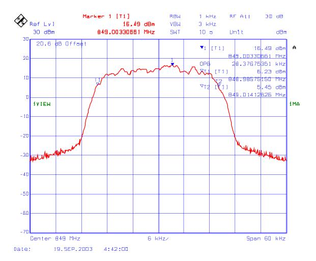
PLOT # 86 99% Occupied Bandwidth- RF Input
