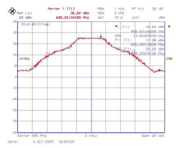
PLOT # 135 99% Occupied Bandwidth- RF Output
