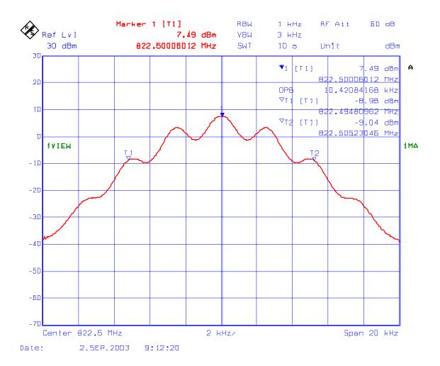
**PLOT #67** 99% Occupied Bandwidth-RF Output
