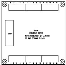
This 4" x 4" Board mounts onto four 3.5" x 3.5" #6 locations, and includes a 6' DB15 to DB15 Cable.
