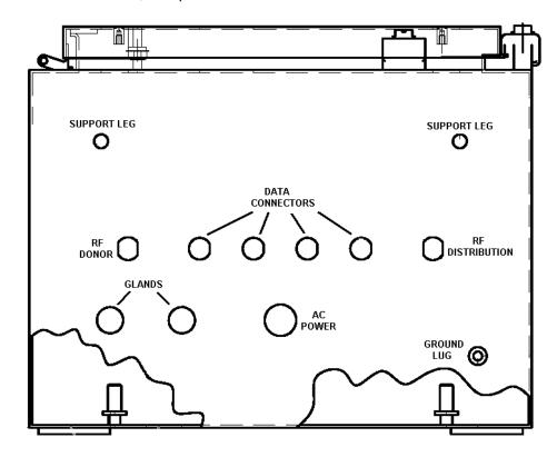
There are openings on the bottoms of the Enclosures for 4 Data Connectors and two of optional SB-GLAND. When not used these openings are sealed with weather-resistant plugs...
