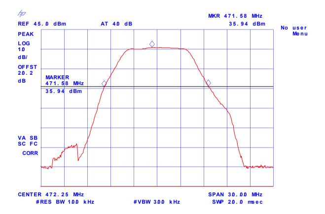
Plot # 13: 99% OBW of RF Input, RF Input Level = 10 dBm as maximum rated by the manufacturer
