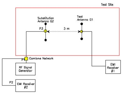
P3 = P2 + Insertian Loss (P1-P3)EIRP = P3 + G2
