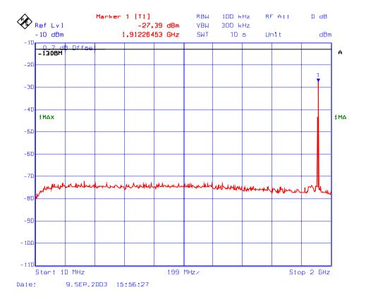
Plot # 207 : Transmitter Conducted Emissions (Multi Input/Output) In 1850–1910 MHz Band Fc: 1909 MHz, Fc - 200 kHz, Fc - 400 kHz, Unmodulated
