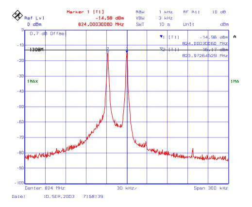
Plot # 9 RF Output Power with 3 RF signal input/output in 806 – 824 MHz Fc: 824 MHz, Fc - 25 kHz, Fc - 50 kHz RF Input 1: -49.50 dBm, RF Input 2: -49.50 dBm, RF Input 3: -49.50 dBm
