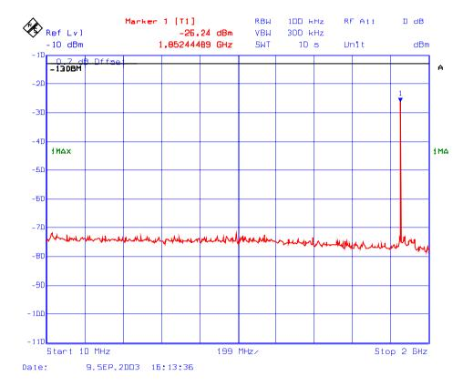
Plot # 199 : Transmitter Conducted Emissions (Multi Input/Output) In 1850–1910 MHz Band Fc: 1851 MHz, Fc + 200 kHz, Fc + 400 kHz, Unmodulated
