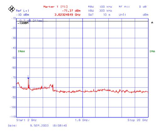
5.10.5.4.14. Uplink Band 1850 - 1910 MHz: Test Frequencies: 1908.8 & 1909 MHz, Modulation: unmodulated (for worst case)
