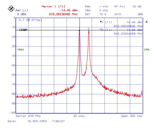
Plot # 6 RF Output Power with 3 RF signal input/output in 806 – 824 MHz Fc: 815 MHz, Fc + 25 kHz, Fc - 25 kHz RF Input 1: -49.50 dBm, RF Input 2: -49.50 dBm, RF Input 3: -49.50 dBm
