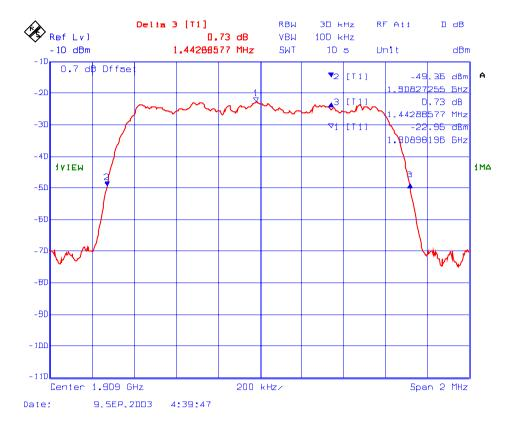
Plot # 84 : 26 dB BW of the 1850 – 1910 MHz, RF Input
