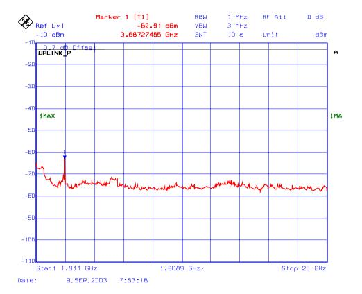
Plot # 186: Transmitter Conducted Emissions Outside the Permitted Band Frequency: 1880 MHz, Modulation: TDMA
