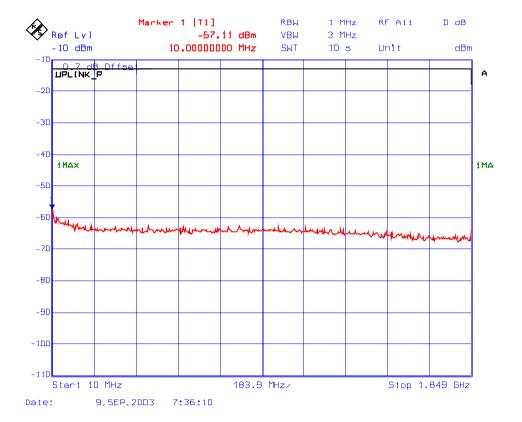
Plot # 193: Transmitter Conducted Emissions Outside the Permitted Band Frequency: 1880 MHz, Modulation: GSM
