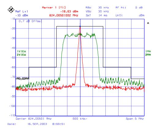
Plot # 118 : Emission Mask CDMA, RF Output Frequency: 836.5 MHz, Modulation: CDMA
