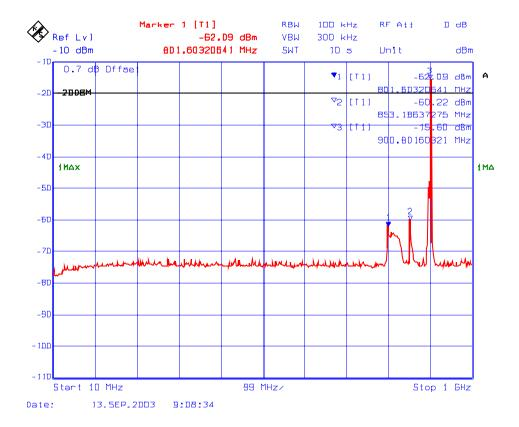
Plot # 177 : Transmitter Spurious Emissions Conducted with 3 RF signal input in 896 – 901 MHz
