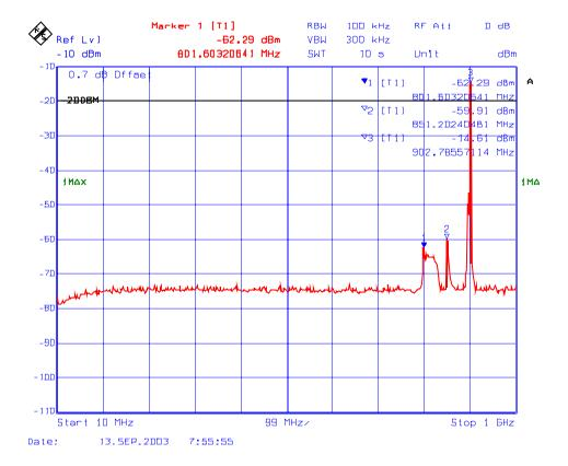
Plot # 173 : Transmitter Spurious Emissions Conducted with 1 RF signal input in 896 – 901 MHz
