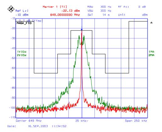
Plot # 116: Emission Mask CDMA, RF Input Frequency: 836.5 MHz, Modulation: CDMA
