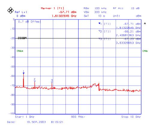
Plot # 134 : Transmitter Spurious Emissions Conducted with 3 RF signal input in 806 – 824 MHz
