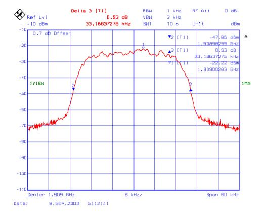
Plot # 88 : 26 dB BW of the 1850 – 1910 MHz, RF Input
