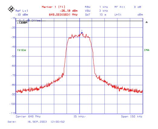
Plot # 122 : Lower Band-Edge, RF Output Frequency: 824 MHz, Modulation: GSM
