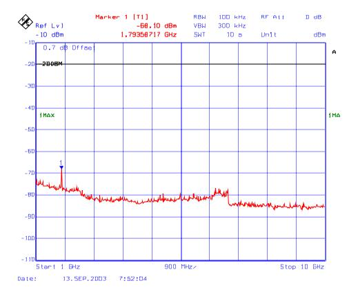
Plot # 174 : Transmitter Spurious Emissions Conducted with 2 RF signal input in 896 – 901 MHz
