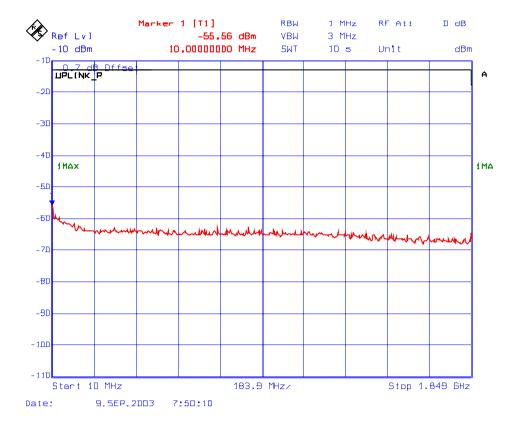
Plot # 187: Transmitter Conducted Emissions Outside the Permitted Band Frequency: 1880 MHz, Modulation: TDMA
