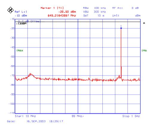
Plot # 163: Transmitter Spurious Emissions Conducted with 2 RF signal input in 824 – 849 MHz
