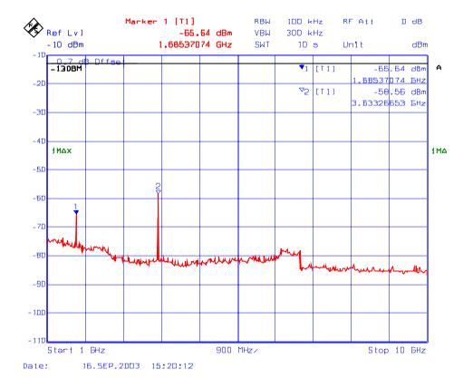
Plot # 162 : Transmitter Spurious Emissions Conducted with 2 RF signal input in 824 – 849 MHz
