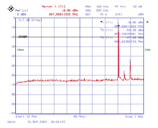
Plot # 135 : Transmitter Spurious Emissions Conducted with 3 RF signal input in 806 – 824 MHz
