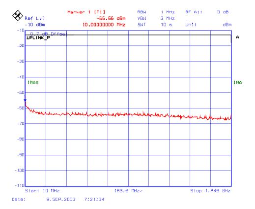
Plot # 183: Transmitter Conducted Emissions Outside the Permitted Band Frequency: 1909 MHz, Modulation: CDMA
