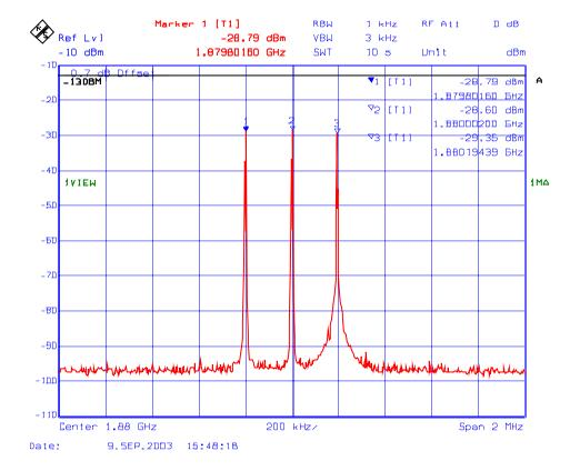
Plot #31 RF Output Power with 1 RF signal input/output in 1850 – 1910 MHz Fc: 1909 MHz, RF Input: -40 dBm
