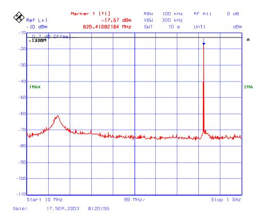
Plot # 153: Transmitter Spurious Emissions Conducted with 3 RF signal input in 824 - 849 MHz
