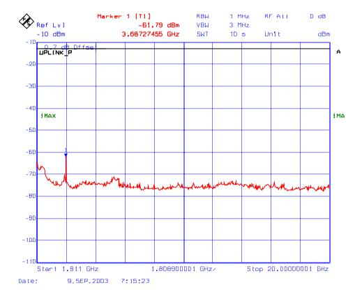
Plot # 180 : Transmitter Conducted Emissions Outside the Permitted Band Frequency: 1880 MHz, Modulation: CDMA
