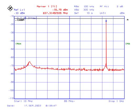
Plot # 159 : Transmitter Spurious Emissions Conducted with 3 RF signal input in 824 – 849 MHz
