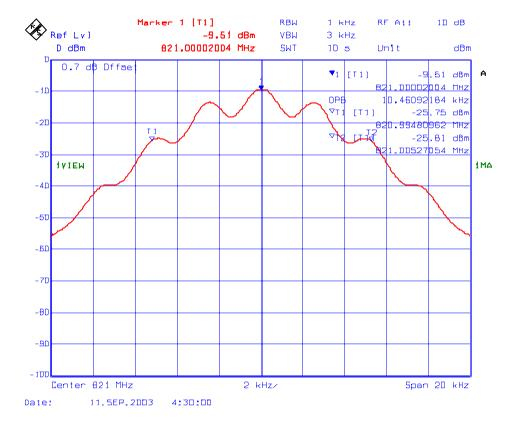
Frequency: 822.5 MHz, 12.5 kHz Channel Spacing
