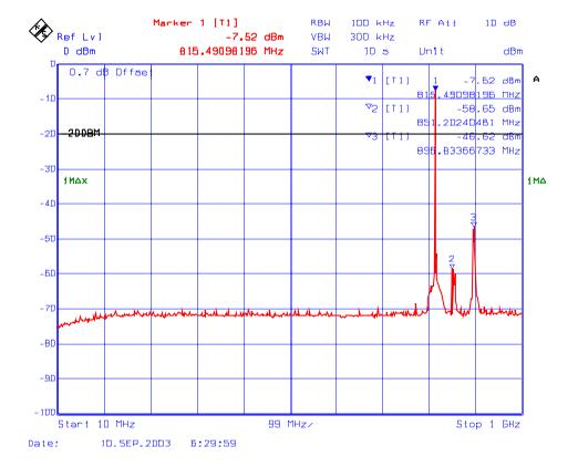
Plot # 137: Transmitter Spurious Emissions Conducted with 1 RF signal input in 806 – 824 MHz
