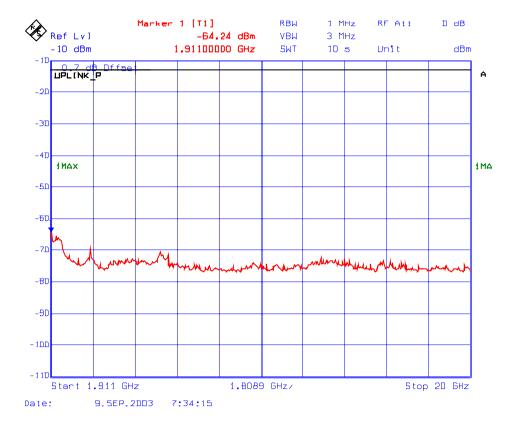
Plot # 194: Transmitter Conducted Emissions Outside the Permitted Band Frequency: 1909 MHz, Modulation: GSM
