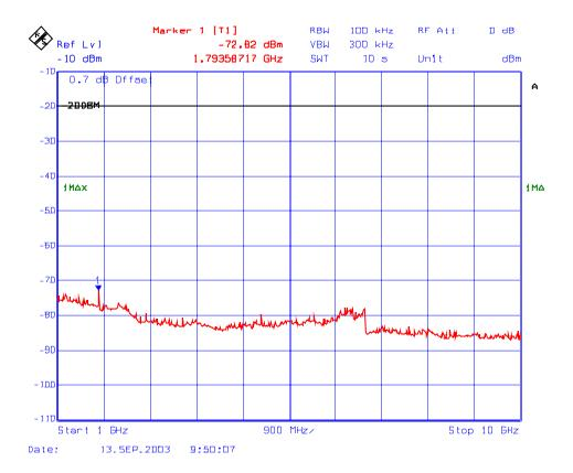
Plot # 170: Transmitter Spurious Emissions Conducted with 3 RF signal input in 896 – 901 MHz
