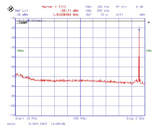
Plot # 205 : Transmitter Conducted Emissions (Multi Input/Output) In 1850–1910 MHz Band Fc: 1909 MHz, Fc - 200 kHz, Unmodulated
