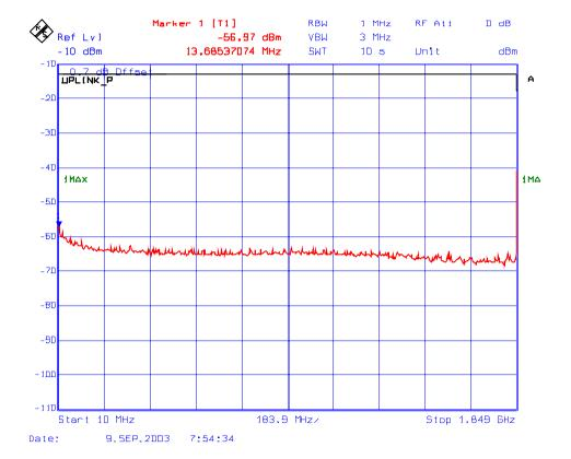
Plot # 185 : Transmitter Conducted Emissions Outside the Permitted Band Frequency: 1851 MHz, Modulation: TDMA
