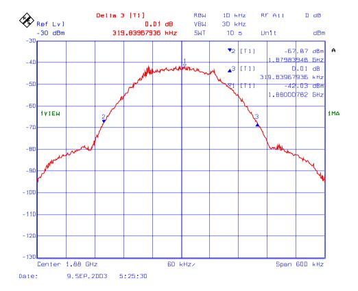
Plot # 89 : 26 dB BW of the 1850 – 1910 MHz, RF Output
