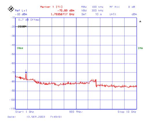
Plot # 168: Transmitter Spurious Emissions Conducted with 2 RF signal input in 896 – 901 MHz
