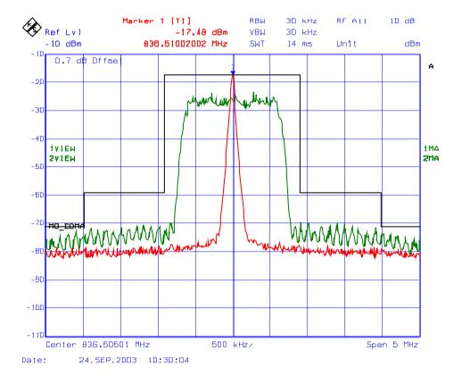
Plot # 119 : Emission Mask CDMA, RF Output Frequency: 849 MHz, Modulation: CDMA
