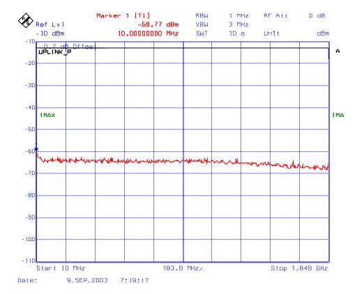
Plot # 181: Transmitter Conducted Emissions Outside the Permitted Band Frequency: 1880 MHz, Modulation: CDMA
