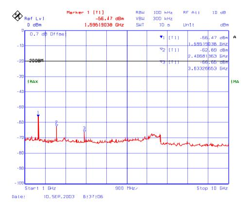
Plot # 132 : Transmitter Spurious Emissions Conducted with 2 RF signal input in 806 – 824 MHz
