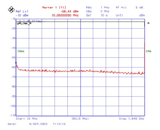
Plot # 179: Transmitter Conducted Emissions Outside the Permitted Band Frequency: 1851 MHz, Modulation: CDMA
