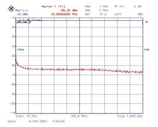
Plot # 191: Transmitter Conducted Emissions Outside the Permitted Band Frequency: 1851 MHz, Modulation: GSM
