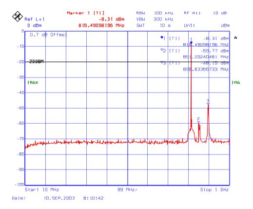
Plot # 139 : Transmitter Spurious Emissions Conducted with 2 RF signal input in 806 – 824 MHz
