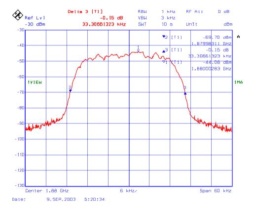
Plot # 85 : 26 dB BW of the 1850 – 1910 MHz, RF Output
