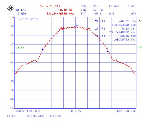
Plot # 91: 26 dB BW of the 1850 – 1910 MHz, RF Output Frequency: 1909 MHz, Modulation: GSM
