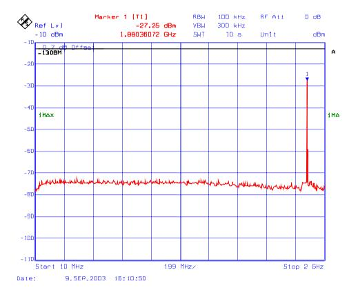
Plot # 203 : Transmitter Conducted Emissions (Multi Input/Output) In 1850–1910 MHz Band Fc: 1880 MHz, Fc - 200 kHz, Fc + 200 kHz, Unmodulated
