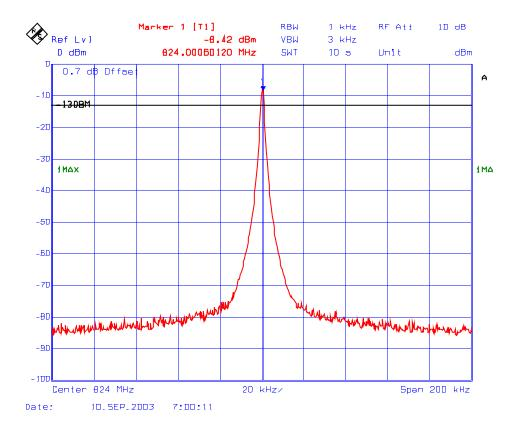
Plot # 8 RF Output Power with 2 RF signal input/output in 806 – 824 MHz
