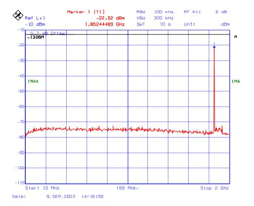
Plot # 197 : Transmitter Conducted Emissions (Multi Input/Output) In 1850–1910 MHz Band Fc: 1851 MHz, Fc + 200 kHz, Unmodulated
