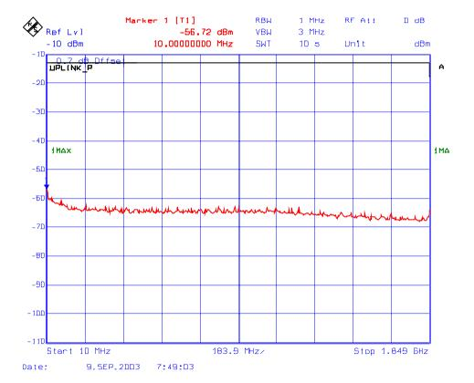
Plot # 189: Transmitter Conducted Emissions Outside the Permitted Band Frequency: 1909 MHz, Modulation: TDMA
