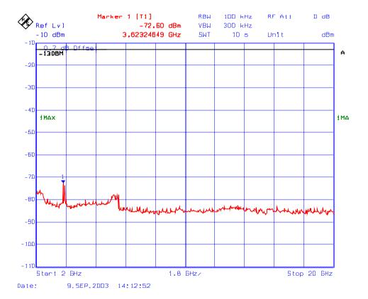
Plot # 202 : Transmitter Conducted Emissions (Multi Input/Output) In 1850–1910 MHz Band Fc: 1880 MHz, Fc - 200 kHz, Fc + 200 kHz, Unmodulated
