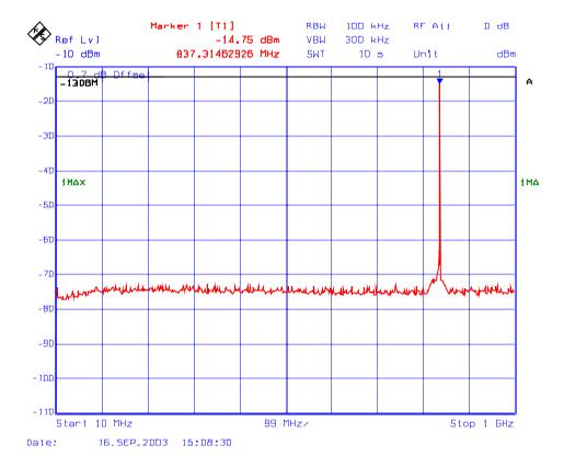
Plot # 155 : Transmitter Spurious Emissions Conducted with 1 RF signal input in 824 - 849 MHz
