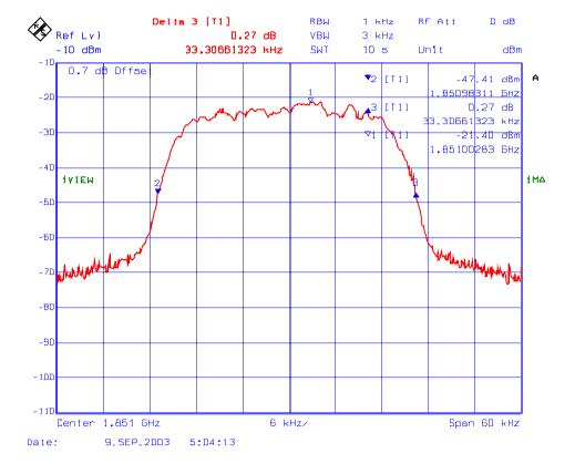
Plot # 86 : 26 dB BW of the 1850 – 1910 MHz, RF Output Frequency: 1880 MHz, Modulation: TDMA
