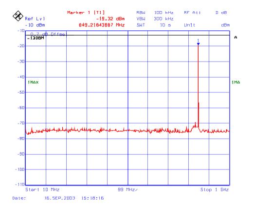
Plot # 161 : Transmitter Spurious Emissions Conducted with 1 RF signal input in 824 - 849 MHz
