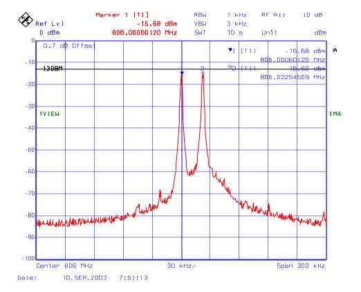
Plot # 3 RF Output Power with 3 RF signal input/output in 806 – 824 MHz Fc: 806 MHz, Fc + 25 kHz, Fc + 50 kHz RF Input 1: -49.50 dBm, RF Input 2: -49.50 dBm, RF Input 3: -49.50 dBm
