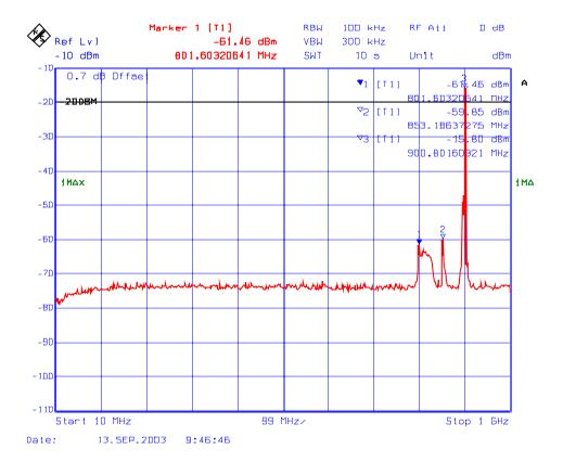
Plot # 175 : Transmitter Spurious Emissions Conducted with 2 RF signal input in 896 – 901 MHz
