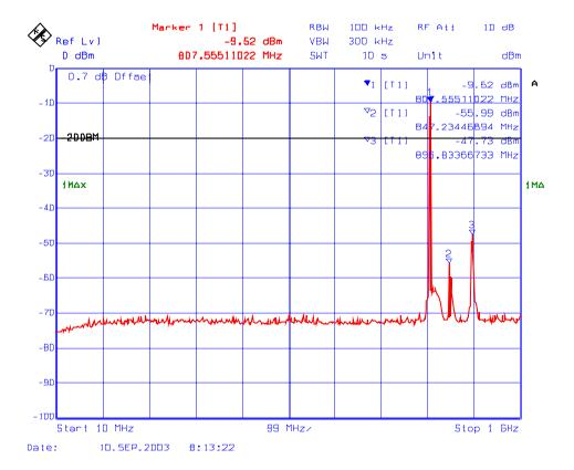
Plot # 133 : Transmitter Spurious Emissions Conducted with 2 RF signal input in 806 – 824 MHz
