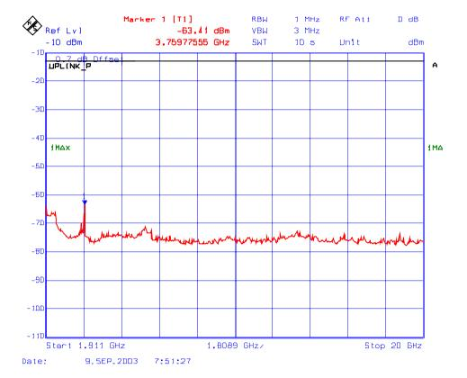
Plot # 188 : Transmitter Conducted Emissions Outside the Permitted Band Frequency: 1909 MHz, Modulation: TDMA
