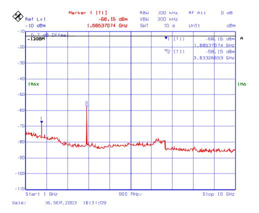
Plot # 164: Transmitter Spurious Emissions Conducted with 3 RF signal input in 824 – 849 MHz
