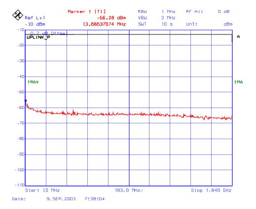
Plot # 195: Transmitter Conducted Emissions Outside the Permitted Band Frequency: 1909 MHz, Modulation: GSM
