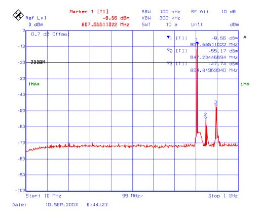
Plot # 131 : Transmitter Spurious Emissions Conducted with 1 RF signal input in 806 - 824 MHz
