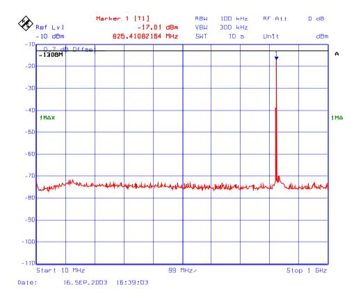
Plot # 151 : Transmitter Spurious Emissions Conducted with 2 RF signal input in 824 – 849 MHz
