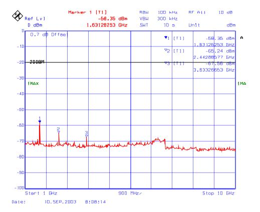
Plot # 140 : Transmitter Spurious Emissions Conducted with 3 RF signal input in 806 – 824 MHz
