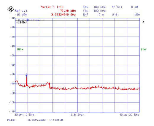
Plot # 198 : Transmitter Conducted Emissions (Multi Input/Output) In 1850–1910 MHz Band Fc: 1851 MHz, Fc + 200 kHz, Fc + 400 kHz, Unmodulated
