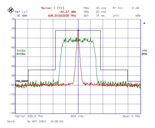
Plot # 117 : Emission Mask CDMA, RF Output Frequency: 824 MHz, Modulation: CDMA
