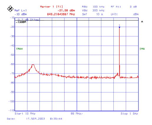
Plot # 165: Transmitter Spurious Emissions Conducted with 3 RF signal input in 824 – 849 MHz
