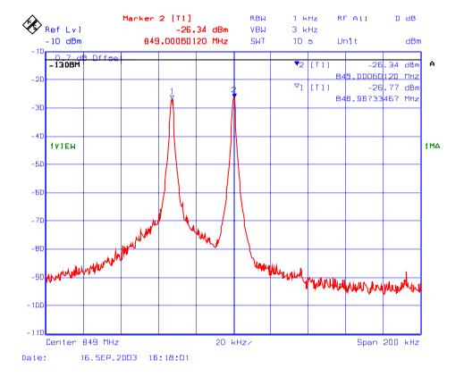
Plot #18 RF Output Power with 3 RF signal input/output in 824 – 849 MHz Fc: 849 MHz, Fc - 30 kHz, Fc - 60 kHz RF Input 1: -42.68 dBm, RF Input 2: -42.68 dBm, RF Input 3: -42.68 dBm
