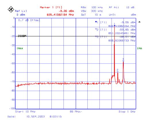
Plot # 145 : Transmitter Spurious Emissions Conducted with 2 RF signal input in 806 – 824 MHz
