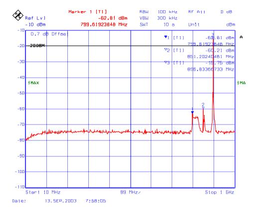
Plot # 167: Transmitter Spurious Emissions Conducted with 1 RF signal input in 896 – 901 MHz
