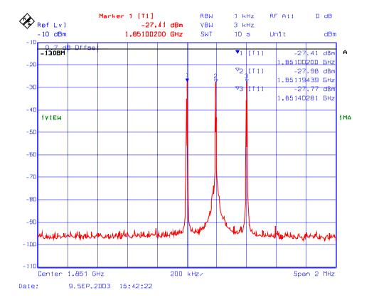
Plot #28 RF Output Power with 1 RF signal input/output in 1850 – 1910 MHz Fc: 1880 MHz, RF Input: -40 dBm
