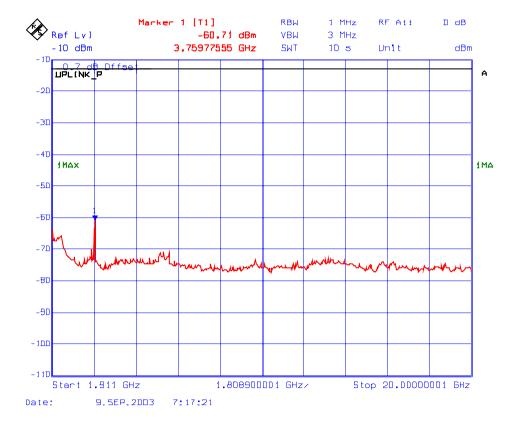
Plot # 182: Transmitter Conducted Emissions Outside the Permitted Band Frequency: 1909 MHz, Modulation: CDMA
