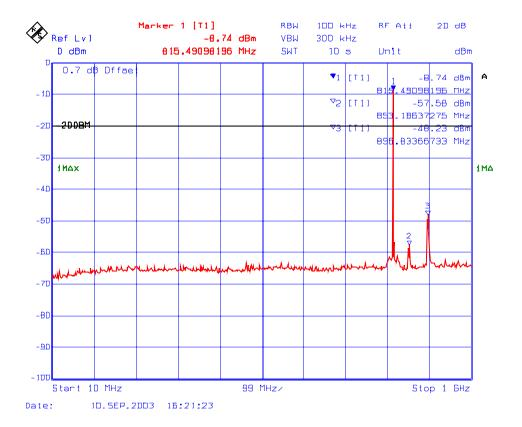
Plot # 141 : Transmitter Spurious Emissions Conducted with 3 RF signal input in 806 – 824 MHz
