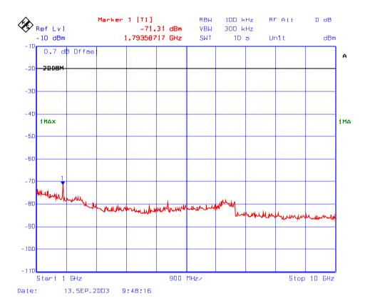
Plot # 176 : Transmitter Spurious Emissions Conducted with 3 RF signal input in 896 – 901 MHz
