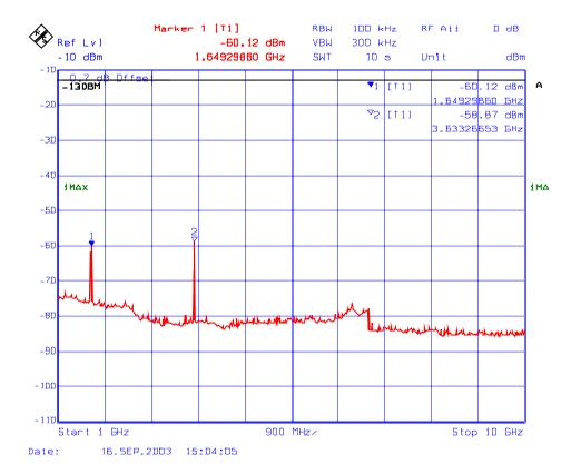
Plot # 150 : Transmitter Spurious Emissions Conducted with 2 RF signal input in 824 – 849 MHz
