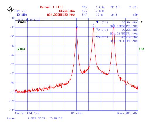
Plot #13 RF Output Power with 1 RF signal input/output in 824 – 849 MHz Fc: 836.5 MHz, RF Input: -40 dBm
