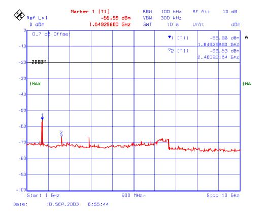
Plot # 144 : Transmitter Spurious Emissions Conducted with 2 RF signal input in 806 – 824 MHz
