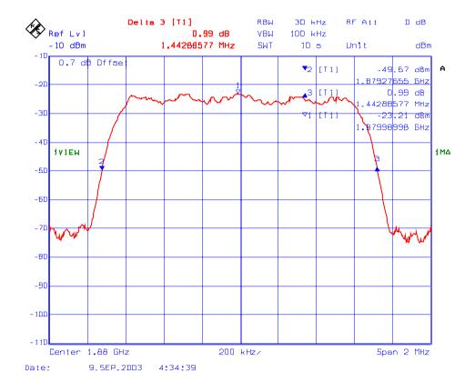
Plot # 83: 26 dB BW of the 1850 – 1910 MHz, RF Output Frequency: 1909 MHz, Modulation: CDMA
