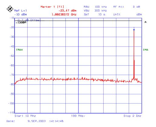
Plot # 201 : Transmitter Conducted Emissions (Multi Input/Output) In 1850–1910 MHz Band Fc: 1880 MHz, Fc + 200 kHz, Unmodulated
