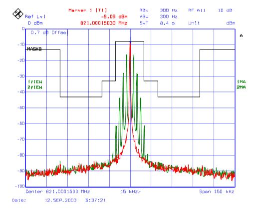
Plot # 94 : Emission Mask B, RF Output Signal
