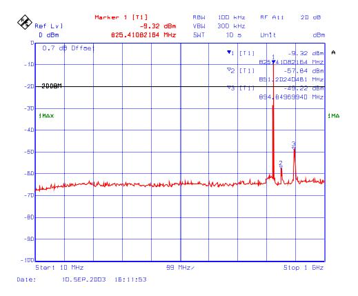
Plot # 147 : Transmitter Spurious Emissions Conducted with 3 RF signal input in 806 – 824 MHz
