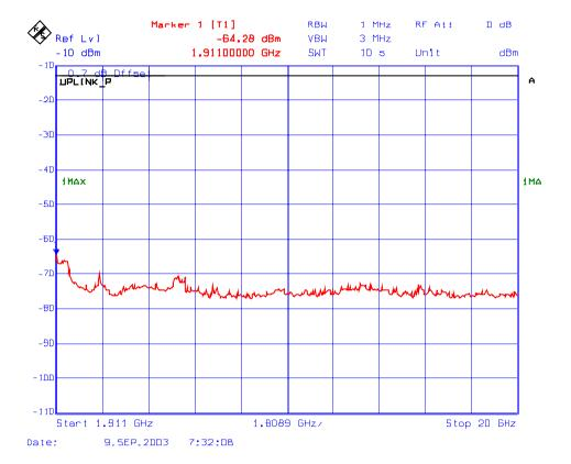
Plot # 192: Transmitter Conducted Emissions Outside the Permitted Band Frequency: 1880 MHz, Modulation: GSM
