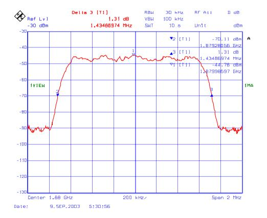
Plot # 81: 26 dB BW of the 1850 – 1910 MHz, RF Output Frequency: 1851 MHz, Modulation: CDMA
