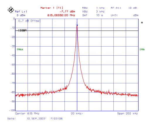
Plot # 5 RF Output Power with 2 RF signal input/output in 806 – 824 MHz
