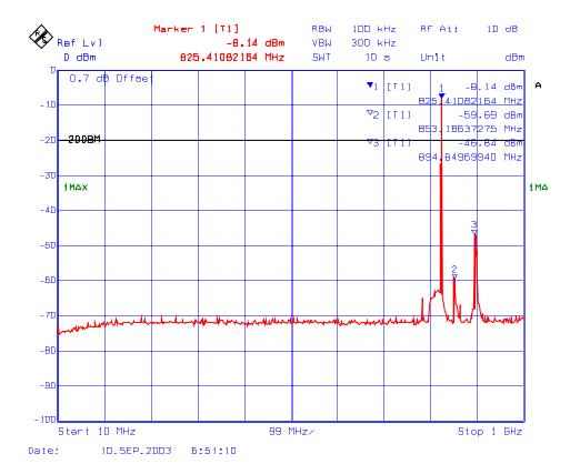
Plot # 143 : Transmitter Spurious Emissions Conducted with 1 RF signal input in 806 – 824 MHz
