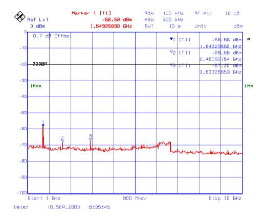
Plot # 146 : Transmitter Spurious Emissions Conducted with 3 RF signal input in 806 – 824 MHz
