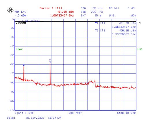
Plot # 158 : Transmitter Spurious Emissions Conducted with 3 RF signal input in 824 – 849 MHz
