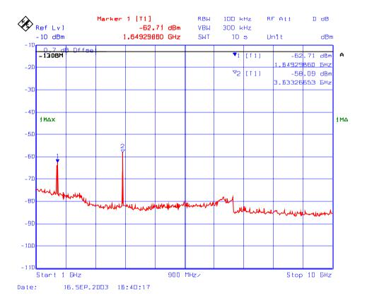
Plot # 152 : Transmitter Spurious Emissions Conducted with 3 RF signal input in 824 – 849 MHz
