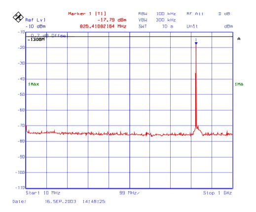
Plot # 149 : Transmitter Spurious Emissions Conducted with 1 RF signal input in 824 - 849 MHz
