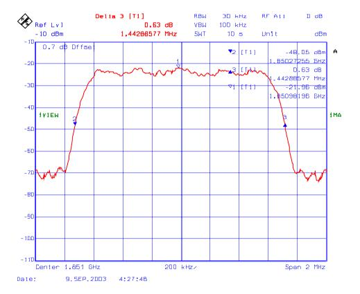
Plot # 82: 26 dB BW of the 1850 – 1910 MHz, RF Output Frequency: 1880 MHz, Modulation: CDMA
