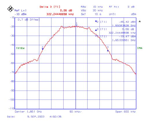
Plot # 90: 26 dB BW of the 1850 – 1910 MHz, RF Output
