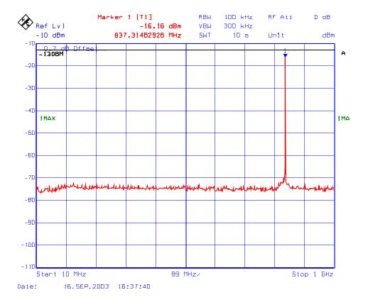
Plot # 157 : Transmitter Spurious Emissions Conducted with 2 RF signal input in 824 – 849 MHz
