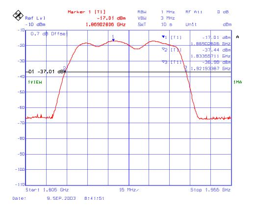
Plot # 80 : 26 dB BW of the 1850 – 1910 MHz, RF Input
