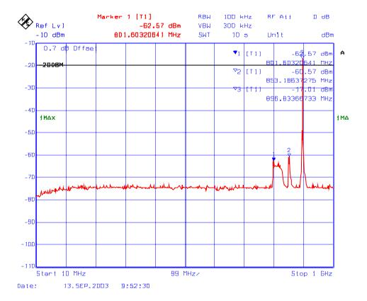
Plot # 169: Transmitter Spurious Emissions Conducted with 2 RF signal input in 896 – 901 MHz
