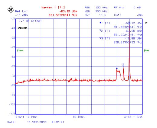
Plot # 171: Transmitter Spurious Emissions Conducted with 3 RF signal input in 896 – 901 MHz
