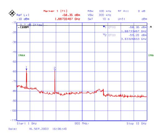
Plot # 156 : Transmitter Spurious Emissions Conducted with 2 RF signal input in 824 – 849 MHz
