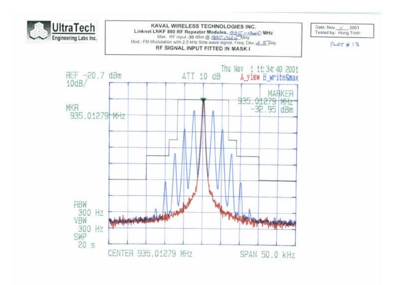
Photo # 14 EMISSION MASKS - FM Modulation with Voice Signal
