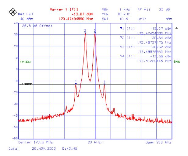
PLOT#: 9 Intermodulation with 3 RF signal inputs
