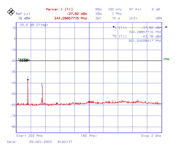
PLOT #: 56 Transmitter Spurious Emissions Conducted with 2 RF signal input Fc: 173.5 MHz, Fc - 12.5 kHz
