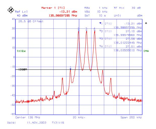
PLOT#: 4 Intermodulation with 1 RF signal input Fc: 160 MHz, RF Input: 3 dBm
