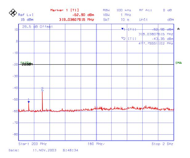
PLOT #: 52 Transmitter Spurious Emissions Conducted with 3 RF signal input Fc: 160 MHz, Fc + 12.5 kHz, Fc – 12.5 kHz
