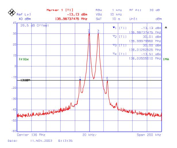
PLOT#: 3 Intermodulation with 3 RF signal input Fc: 136 MHz, Fc + 12.5 kHz, Fc + 25 kHz RF Input 1: -7.33 dBm, RF Input 2: -7.42 dBm, RF Input 3: -7.51 dBm
