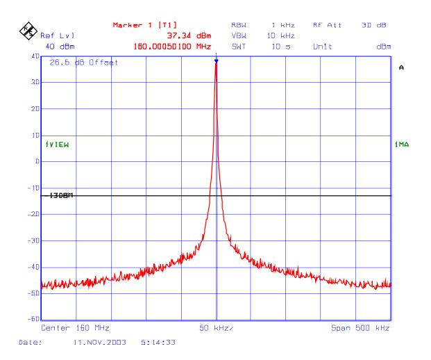
PLOT#: 5 Intermodulation with 2 RF signal inputs Fc: 160 MHz, Fc + 12.5 kHz, RF Input 1: -3.31 dBm, RF Input 2: -3.21 dBm
