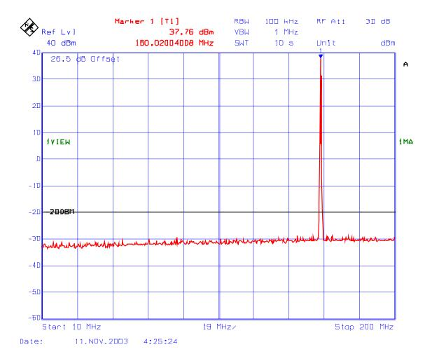
PLOT #: 49 Transmitter Spurious Emissions Conducted with 1 RF signal input Fc: 160 MHz
