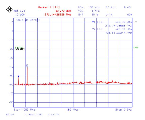
PLOT #: 44 Transmitter Spurious Emissions Conducted with 2 RF signal input Fc: 136 MHz, Fc + 12.5 kHz
