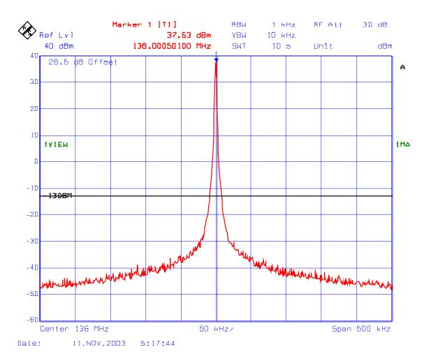
PLOT#: 2 Intermodulation with 2 RF signal input Fc: 136 MHz, Fc + 12.5 kHz, RF Input 1: -4.35 dBm, RF Input 2: -4.41 dBm
