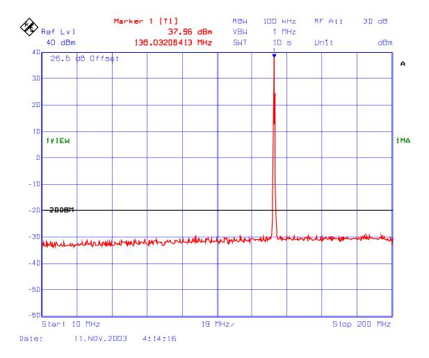
PLOT #: 43 Transmitter Spurious Emissions Conducted with 1 RF signal input Fc: 136 MHz
