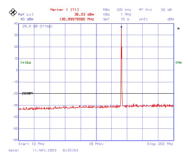
PLOT #: 45 Transmitter Spurious Emissions Conducted with 2 RF signal input Fc: 136 MHz, Fc + 12.5 kHz
