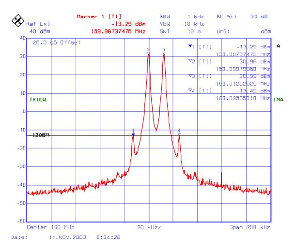
PLOT#: 6 Intermodulation with 3 RF signal inputs
