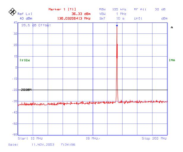
PLOT #: 47 Transmitter Spurious Emissions Conducted with 3 RF signal input Fc: 136 MHz, Fc + 12.5 kHz, Fc + 25 kHz
