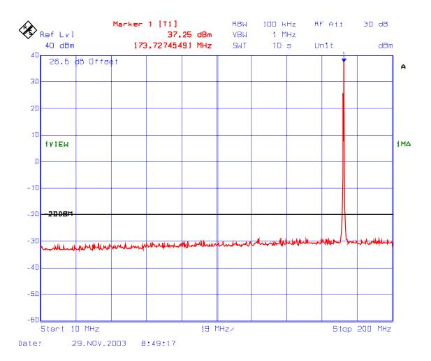
PLOT #: 55 Transmitter Spurious Emissions Conducted with 1 RF signal input Fc: 173.5 MHz
