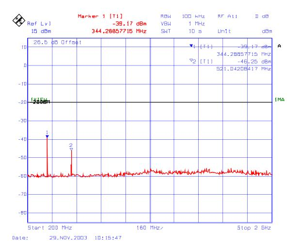
PLOT #: 58 Transmitter Spurious Emissions Conducted with 3 RF signal input Fc: 173.5 MHz, Fc - 12.5 kHz, Fc -25 kHz
