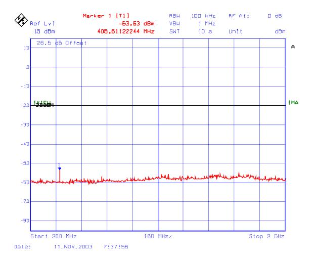
PLOT #: 48 Transmitter Spurious Emissions Conducted with 1 RF signal input Fc: 160 MHz
