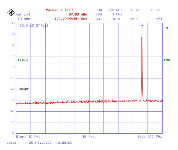
PLOT #: 59 Transmitter Spurious Emissions Conducted with 3 RF signal input Fc: 173.5 MHz, Fc - 12.5 kHz, Fc -25 kHz
