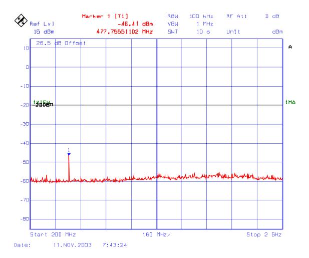
PLOT #: 54 Transmitter Spurious Emissions Conducted with 1 RF signal input Fc: 173.5 MHz
