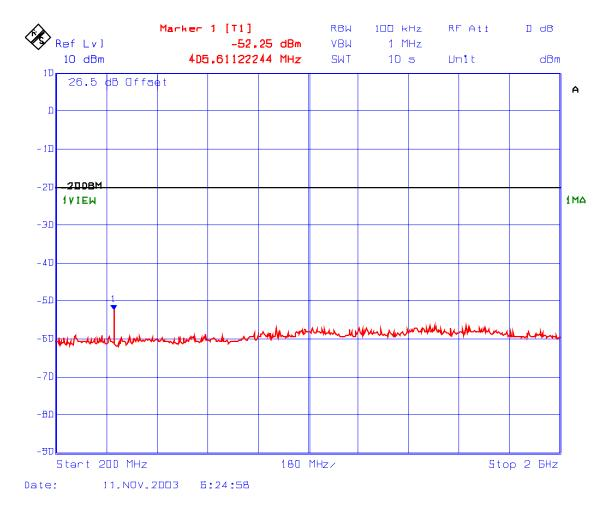
PLOT #: 46 Transmitter Spurious Emissions Conducted with 3 RF signal input Fc: 136 MHz, Fc + 12.5 kHz, Fc + 25 kHz
