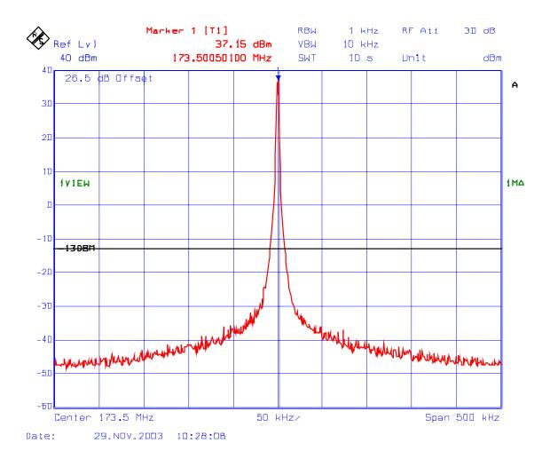
PLOT#: 8 Intermodulation with 2 RF signal inputs Fc: 173.5 MHz, Fc - 12.5 kHz RF Input 1: -3.49 dBm, RF Input 2: -3.62 dBm
