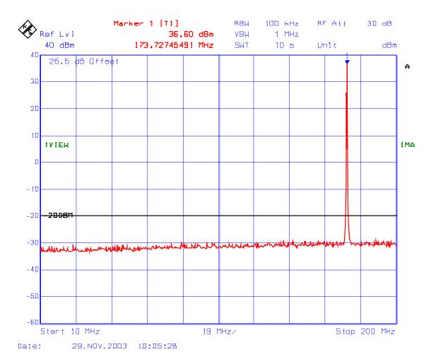
PLOT #: 57 Transmitter Spurious Emissions Conducted with 2 RF signal input Fc: 173.5 MHz, Fc - 12.5 kHz
