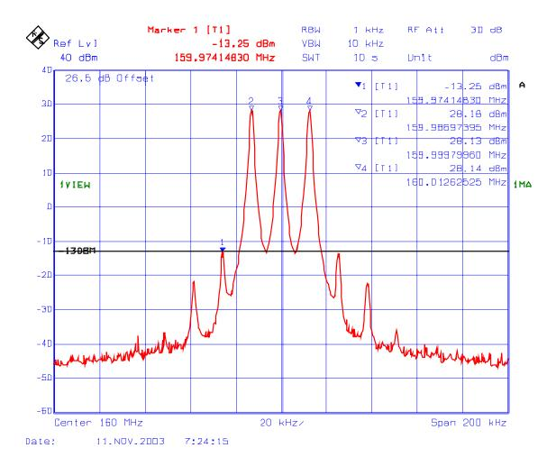
PLOT#: 7 Intermodulation with 1 RF signal input Fc: 173.5 MHz, RF Input: 3 dBm
