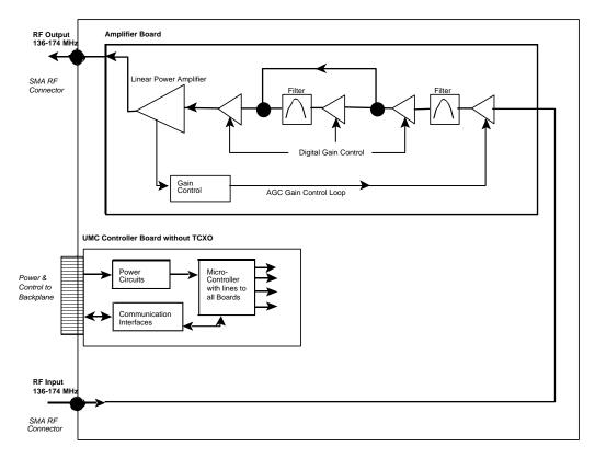
There is no **Tuning** for this product. It is calibrated when it undergoes Factory Testing. When installed the Amplifier is set up by software (see the User Manual) for the desired Gain and AGC setting. The combination of these two settings ensures that the Maximum Power and RF De-Rating requirements are met.
