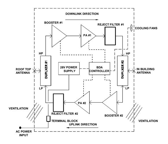
Power and Control Connections RF Connections
