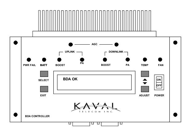
The BDA Controller display is a 2 line by 20 character Vacuum Fluorescent (VFD) display. The connectors are all secure lock types and should only be plugged and unplugged by a service technician.
