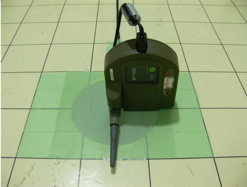
Photograph 8: Set-up for Radiated Emission, EUT Configuration Z-Axis
