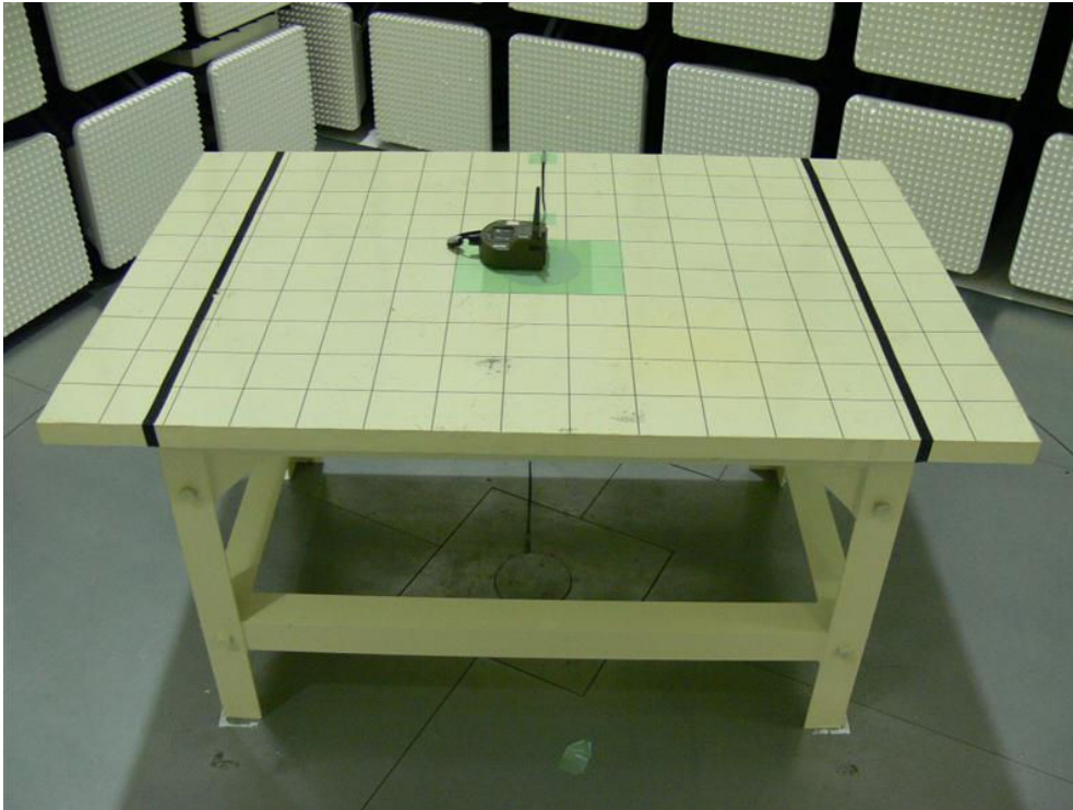
Photograph 4: Set-up for Radiated Emission of Transmitter, Power Input Method “y”, Front View
