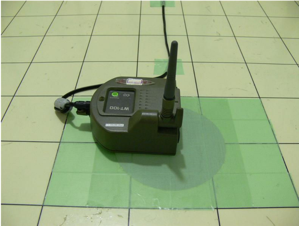
Photograph 6: Set-up for Radiated Emission, EUT Configuration X-Axis
