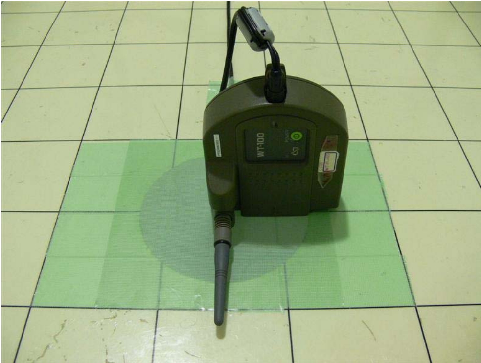
Photograph 8: Set-up for Radiated Emission, EUT Configuration Z-Axis
