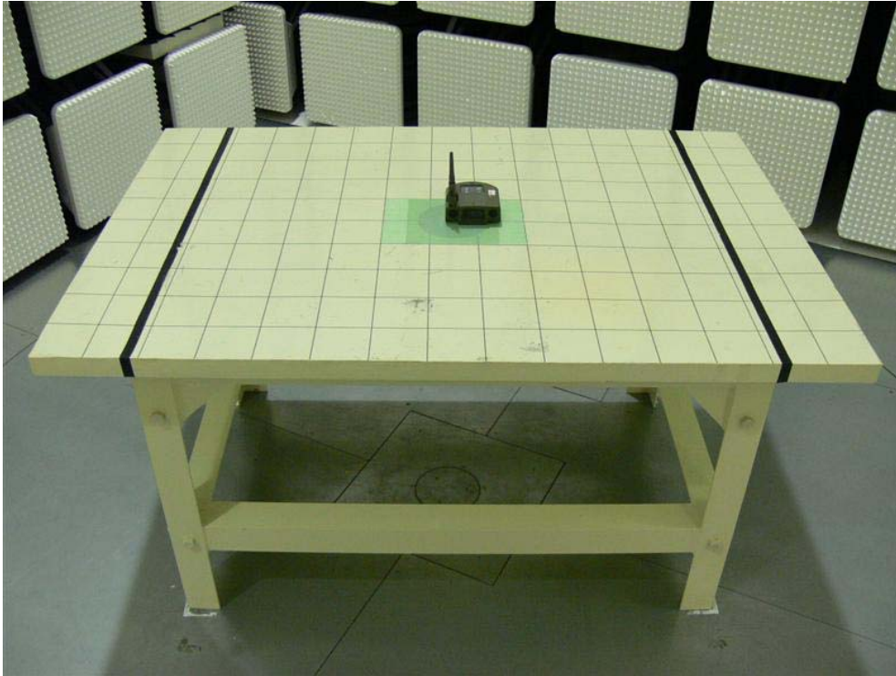
Photograph 2: Set-up for Radiated Emission of Transmitter, Power Input Method "x", Front View
