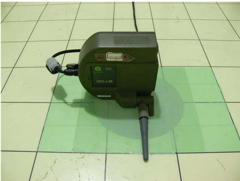
Photograph 7: Set-up for Radiated Emission, EUT Configuration Y-Axis
