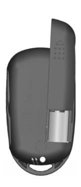
The One-way remote is powered by one CR2032 Battery. To replace battery use a coin or small flat blade screwdriver to carefully pry apart case
