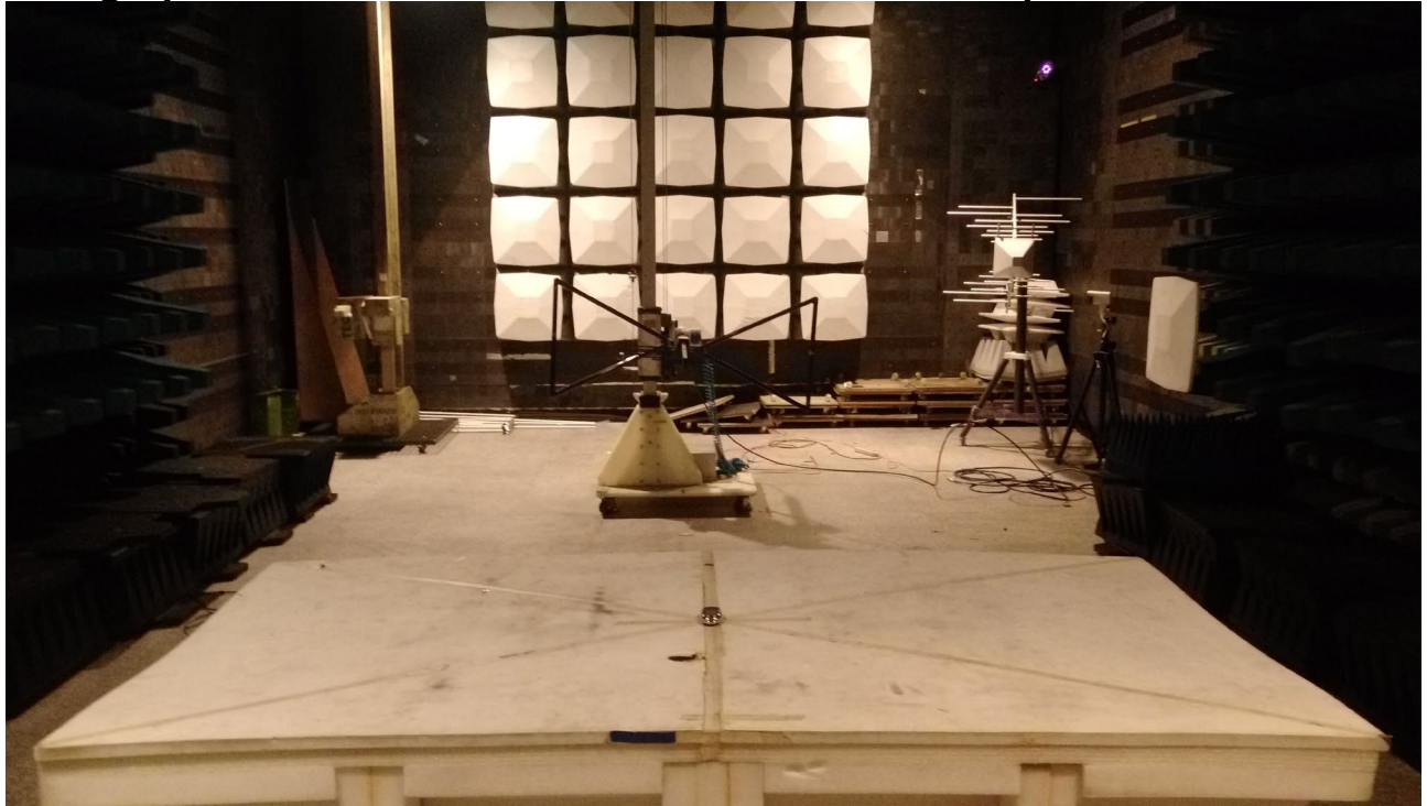
Photograph – Radiated Emission Below 1G Test Setup
