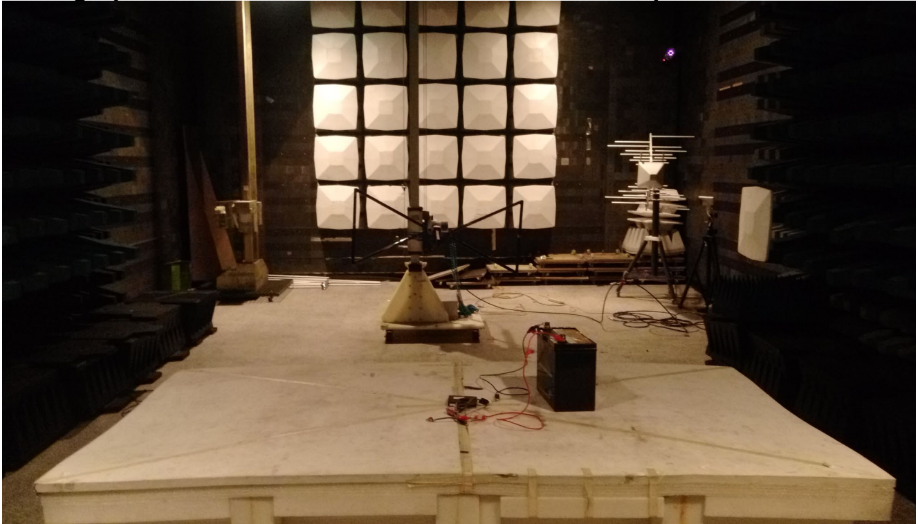
Photograph – Radiated Emission Below 1G Test Setup
