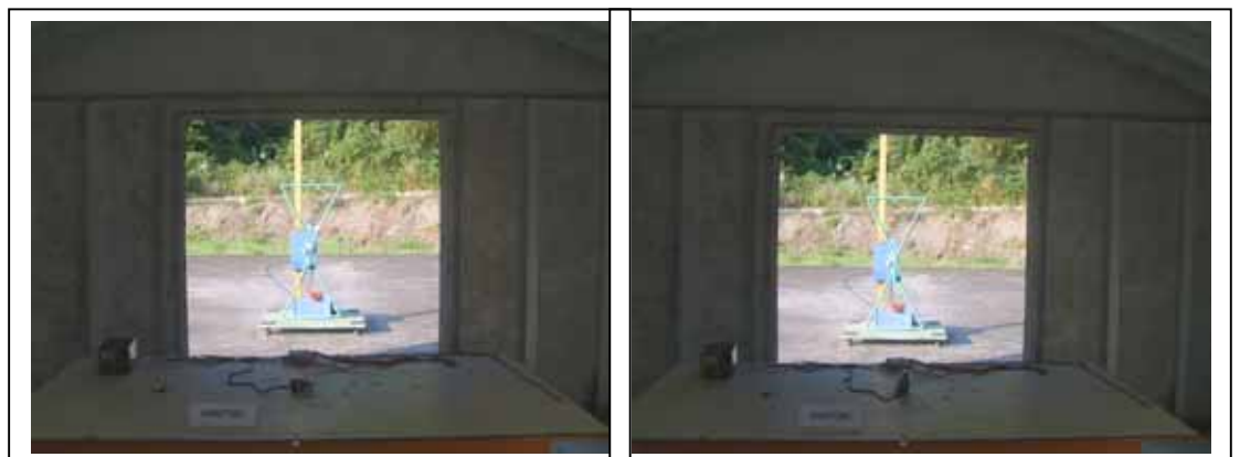
Radiated Open Site Test Set-up
