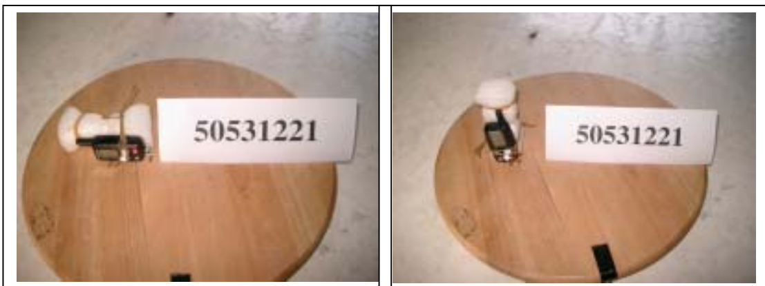
Radiated Open Site Test Set-up
